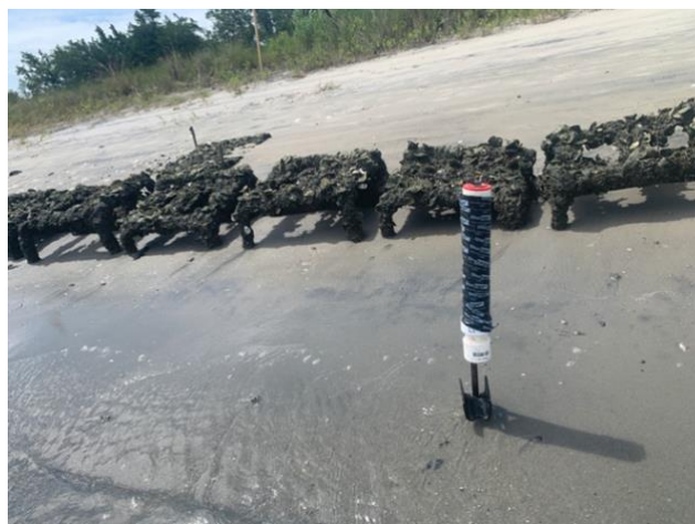
Figure 6: Placement of wave gauge in front of reef, mounted vertically with sensor facing downward (Photo credit: Anna Albright)
