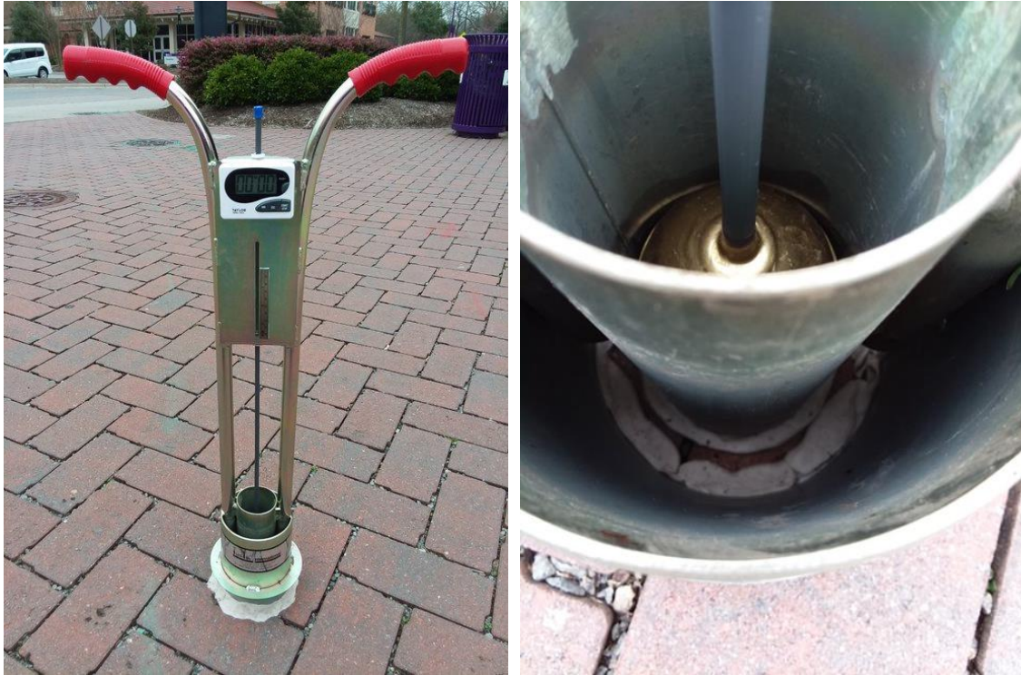
Figure 5. Typical setup of double-ring infiltrometer at PICP test sites.
