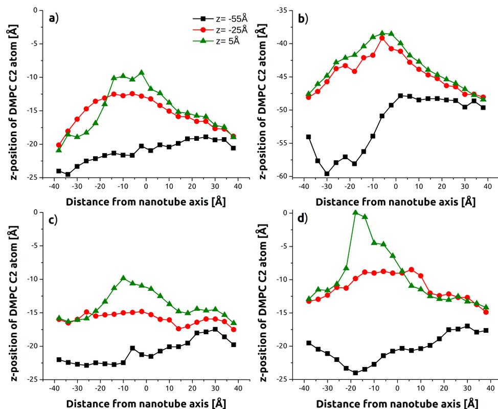
**Figure 8.** Sequential deflection profiles for SiCNT as illustrated by the average DMPC backbone C2 atom position to a resolution of  $4 \text{ \AA}$ . (a) Low rate ( $v = 0.5 \text{ m/s}$ ), tube-axis, upper layer; (b) Low rate ( $v = 0.5 \text{ m/s}$ ), tube-axis, bottom layer; (c) High rate ( $v = 2.0 \text{ m/s}$ ), tube-axis; (d) Low rate ( $v = 0.5 \text{ m/s}$ ), z-axis.
