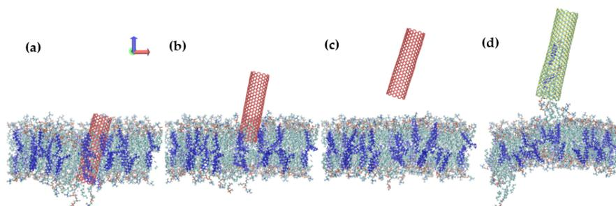
**Figure 6.** A series of snapshots visualizing tube-axis membrane withdrawal for CNT,  $15^\circ$ , and  $v = 2.0$  m/s. Cholesterol molecules inside the DMPC membrane are colored dark blue. (a) CNT indenter at  $z = -55$  Å, (b)  $z = -25$  Å, (c)  $z = 5$  Å; (d) SiCNT indenter at  $z = 5$  Å.
