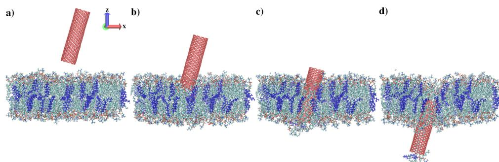
**Figure 1.** A series of snapshots visualizing tube-axis membrane indentation for CNT,  $15^\circ$ , and  $v = 2.0 \text{ m/s}$ . Cholesterol molecules inside the DMPC membrane are dark blue. (a) CNT initial stage (after equilibration); CNT indenter tip is at: (b)  $z = -25 \text{ \AA}$ , (c)  $z = -55 \text{ \AA}$ , (d)  $z = -85 \text{ \AA}$ .
