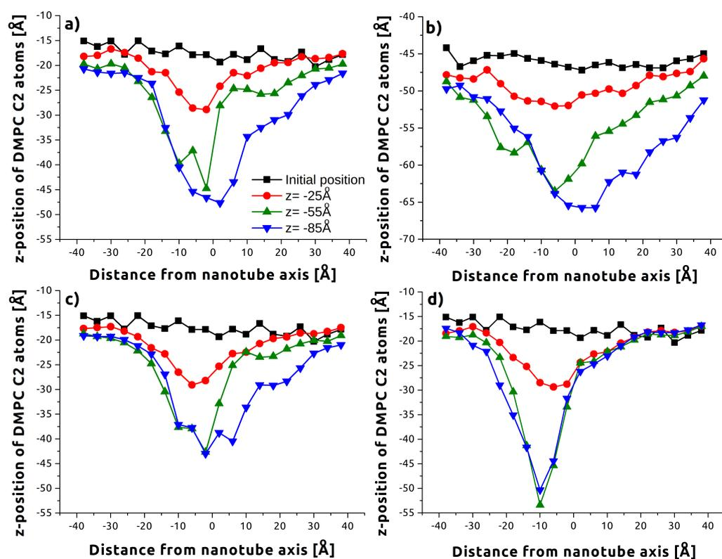
**Figure 5.** Sequential profiles of average DPMC backbone C2 atom position for CNT systems angled at  $15^\circ$  to a resolution of  $4 \text{ \AA}$ . Z-values correspond to the stages shown in Figure 1. Each plot represents a different case: (a)  $z$ -axis indentation at  $2 \text{ m/s}$ —upper layer, (b)  $z$ -axis indentation at  $2 \text{ m/s}$ —lower layer, (c)  $z$ -axis indentation at  $0.5 \text{ m/s}$ —upper layer, (d) tube-axis indentation at  $2 \text{ m/s}$ —upper layer.
