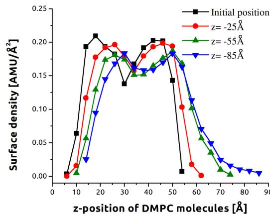
**Figure 3.** The average DMPC mass density profile along the z-axis. Data are for the SiCNT indenter at 2 m/s, a 15° angle z-axis indentation. Each point represents a 4 Å wide average across all equivalent trajectories for the instant specified in the inset.
