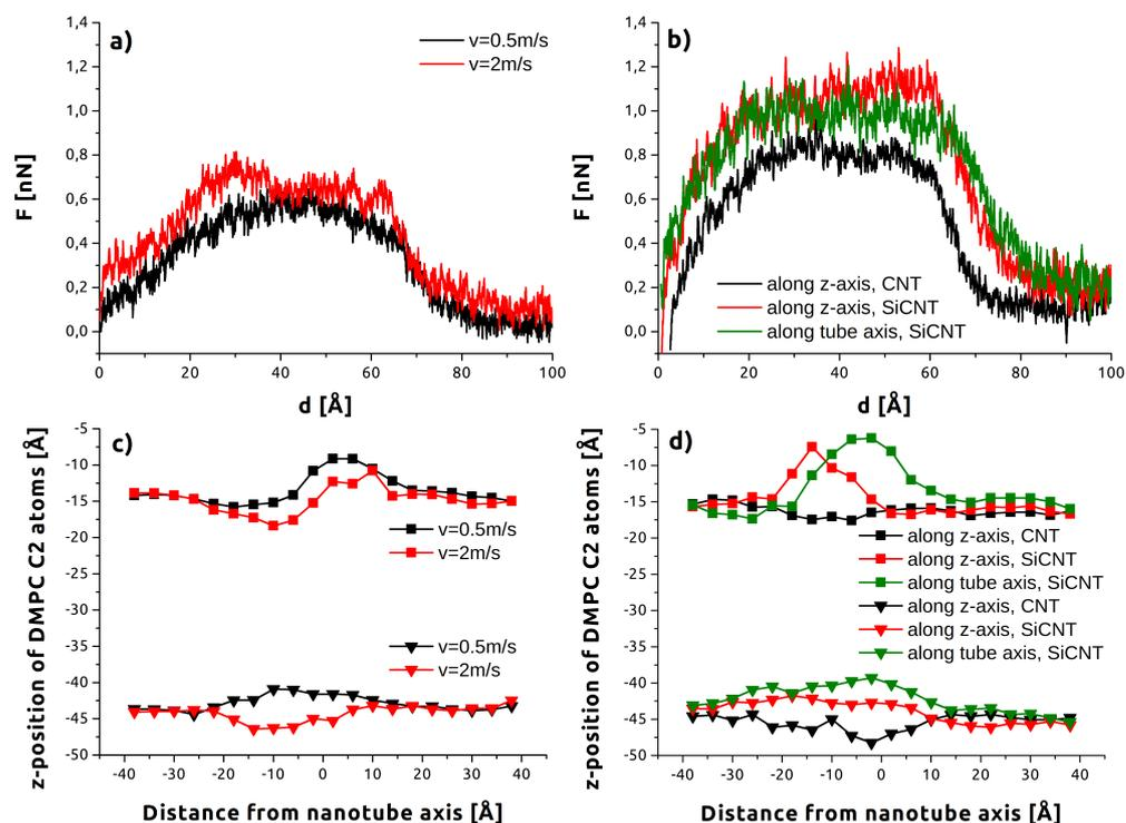
**Figure 7.** SMD forces vs. depth (top row) and backbone C2 atom positions along  $x$ -axis at indenter depth  $d = -25$  Å (bottom): selected comparisons. All cases simulated were angled at  $15^\circ$ . For the C2 atom profiles, both membrane layers are shown. Panels (a,c): rate comparison (CNT, tube-axis indentation). Panels (b,d): nanotube comparison (CNT/SiCNT high rate indentation).
