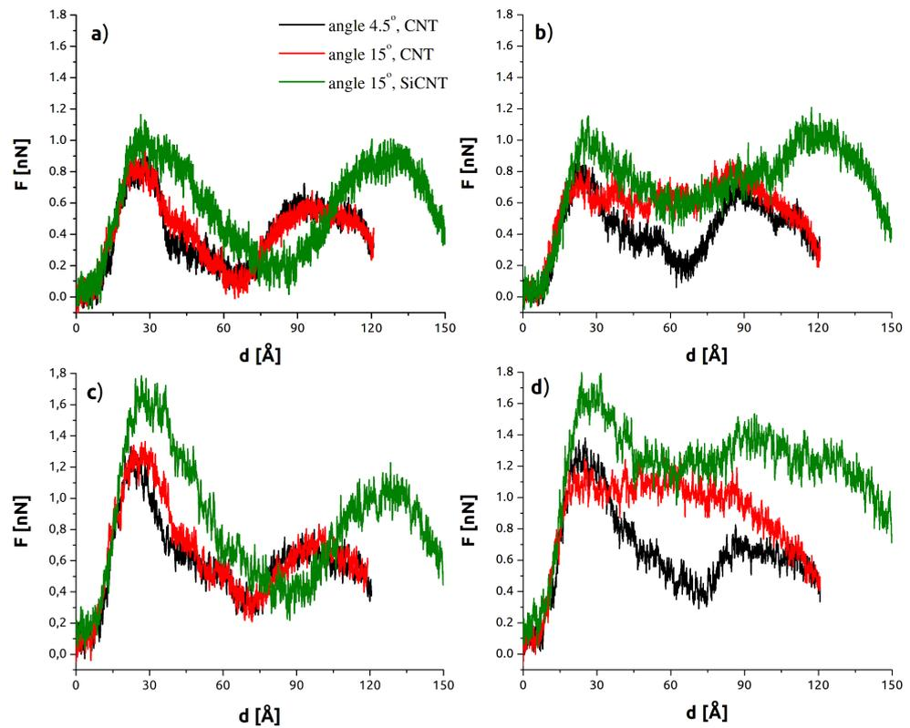
**Figure 2.** SMD force vs. indenter depth. (a) Low rate ( $v = 0.5$  m/s), tube-axis indentation. (b) Low rate ( $v = 0.5$  m/s), z-axis indentation. (c) High rate ( $v = 2.0$  m/s), tube-axis indentation. (d) High rate ( $v = 2.0$  m/s), z-axis indentation.
