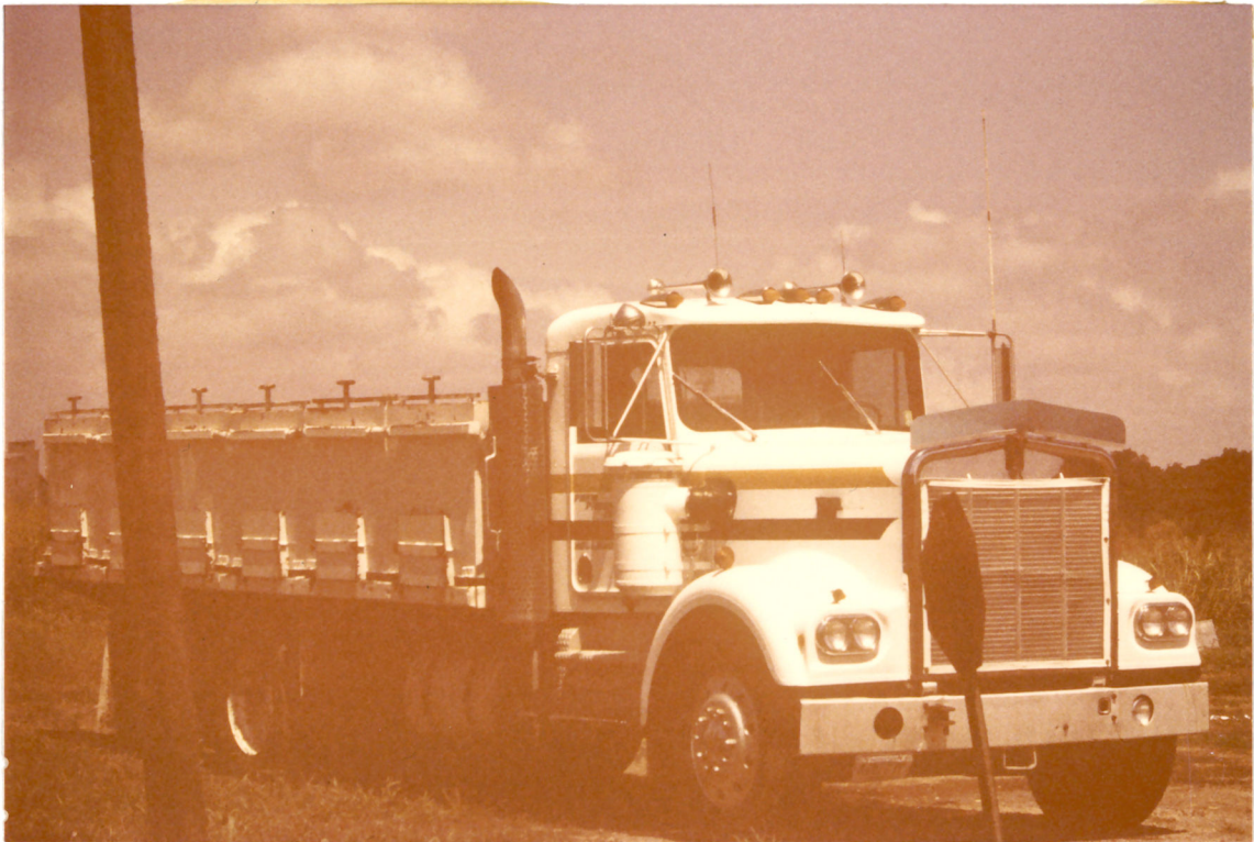
FIGURE 21. This live haul truck is equipped with large aerated water tanks. It is used to haul catfish from ponds to processing plants in Mississippi.
