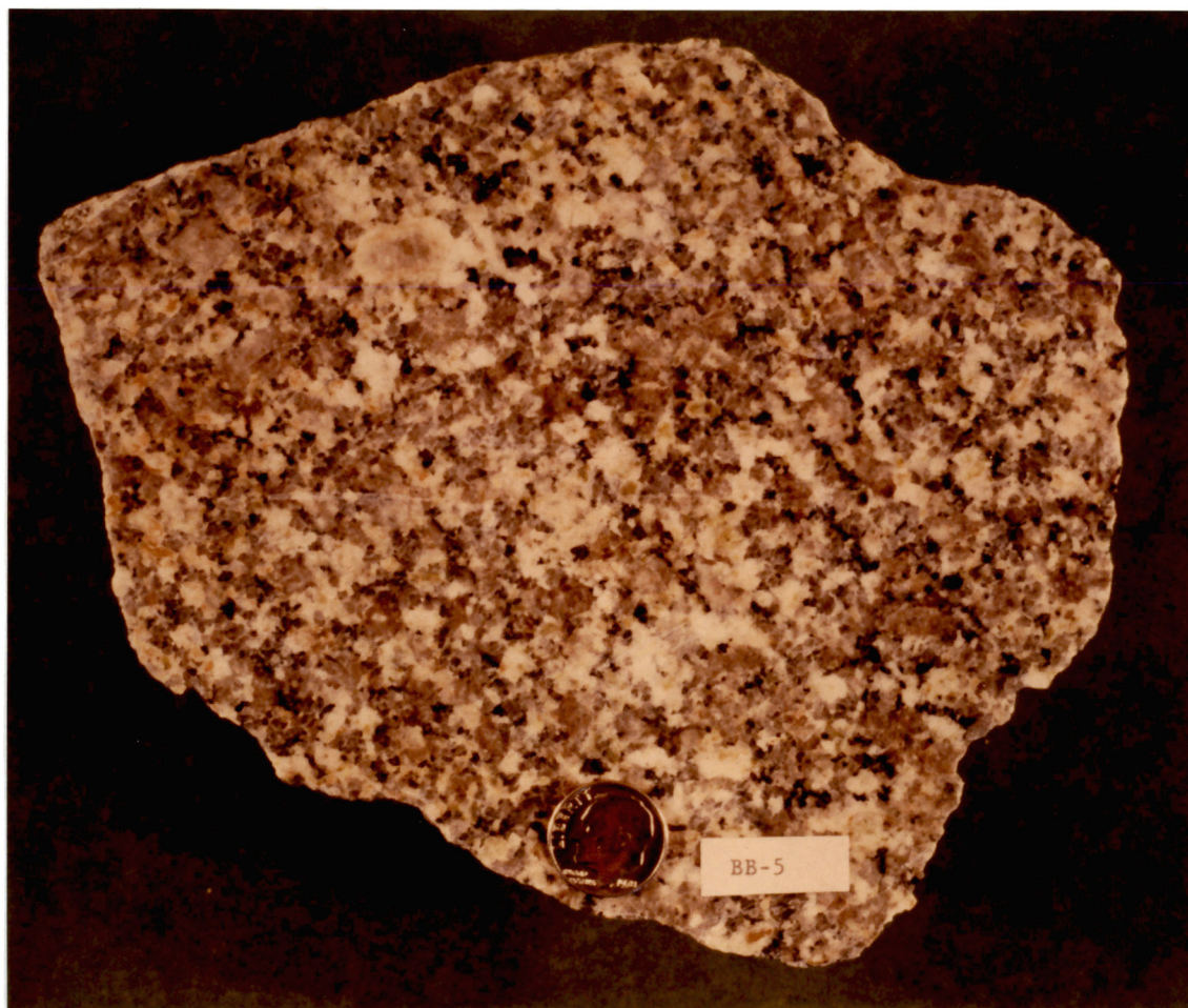
Figure 8. Sample BB-5 showing the typical appearance of fresh granite in the Sims quarry.
