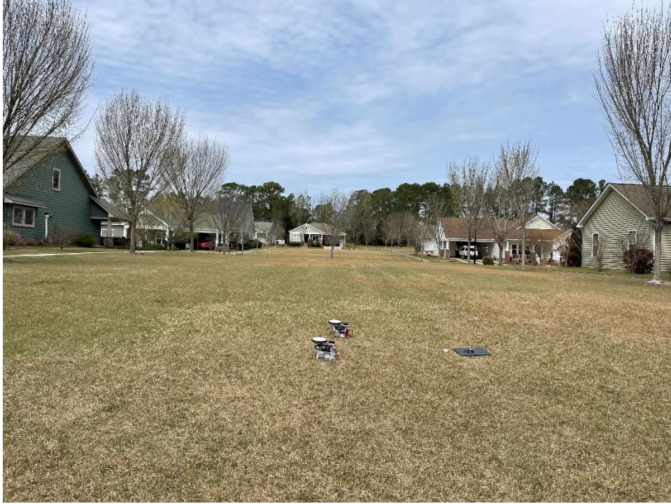
Figure 16. A common data collection location with no obstructions that might hinder the receivers' view of satellites.
