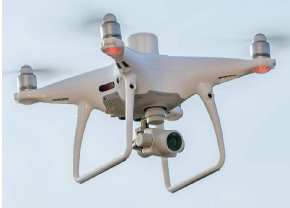
Figure 4. A DJI Phantom 4 Drone with precise relative positioning capability [4].
