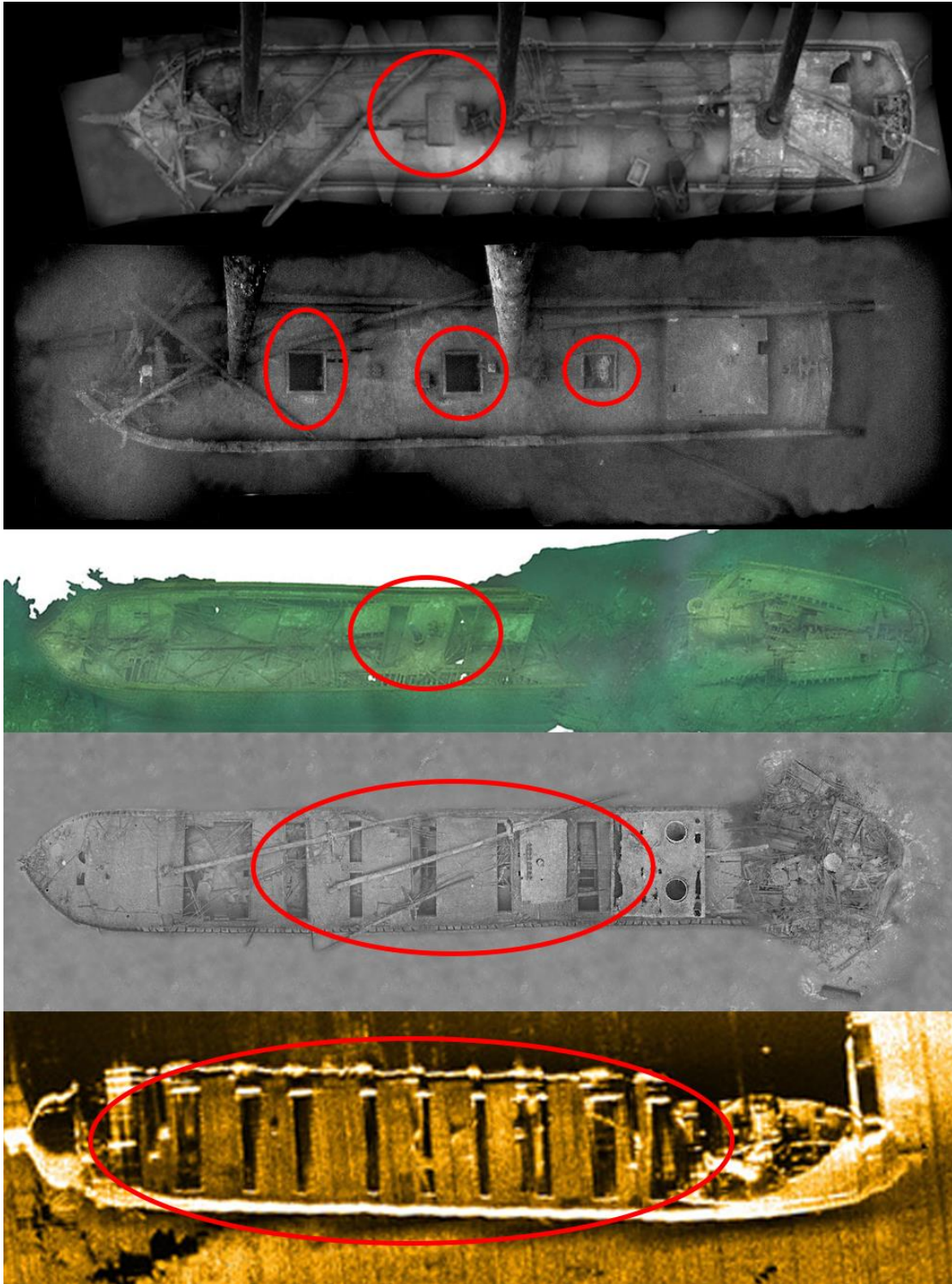
Figure 87: Missing cargo hatches seems to be the norm for intact wrecks in TBNMS (from top to bottom: Cornelia B. Windiate, Kyle Spangler, New Orleans, Florida, and W.C. Franz) (Images by TBNMS; Compiled by Caleb O'Brien).
