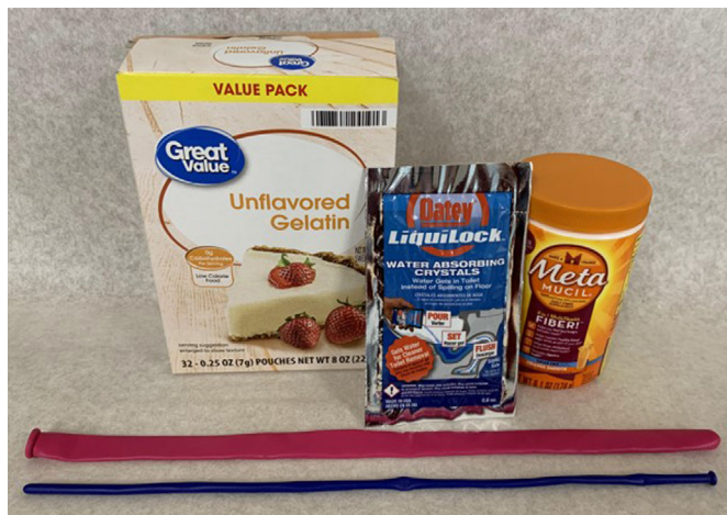
Figure 2: Supplies needed for making the aortic phantoms: 160 and 360 balloons, water-absorbing gel crystals, unflavored gelatin and sugar-free psyllium hydrophilic mucilloid fibre.
