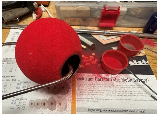
Figure 7: Sifting vitreous enamel onto copper vessel
