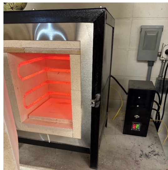
Figure 6: Kiln used for firing vitreous enamel
