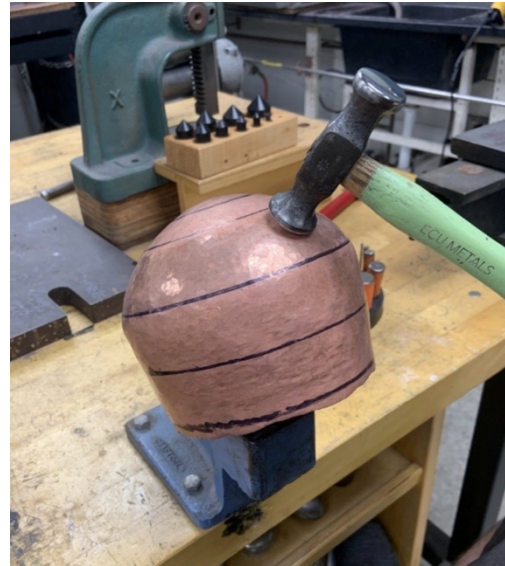
Figure 1: Raised vessel being planished
