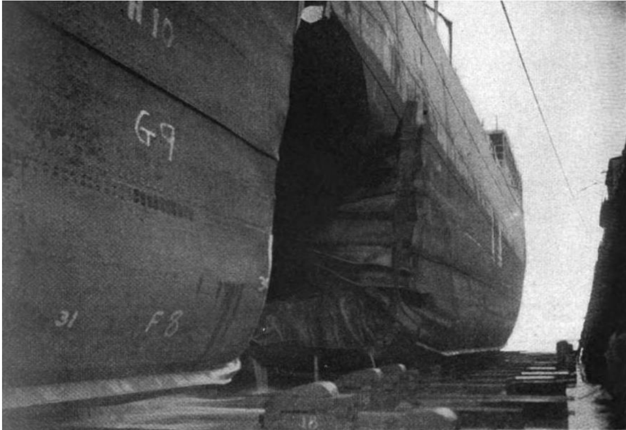
FIGURE 2.7. Hull of the oil tanker Paul H. Harwood after being torpedoed by a U-boat on 7 July 1942. The breach measures 20 by 30 feet, approximately the same size as the hole U-701 's torpedo made in Rockefeller (Standard Oil 1946).
