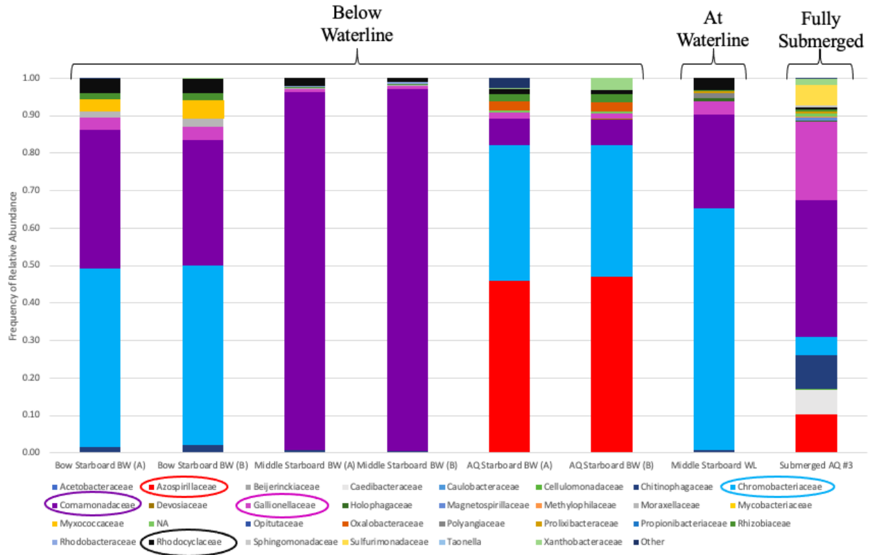
Figure 3: Frequency of relative abundance of present microorganisms in sequenced DNA classified by taxa (family). Samples FeO1 and FeO6 were collected 2.5m into the bow of the starboard at levels below the waterline (BW). FeO2 and FeO7 were collected from 28m into the middle of the starboard below the waterline. FeO3 and FeO8 were collected 54.5m into the after-quarters (AQ) of the starboard side at levels below the waterline. FeO4 was collected 28.5m into the middle of the starboard at the waterline (WL). FeO5 was collected from a fully submerged section of the ship in the after-quarters sector.
