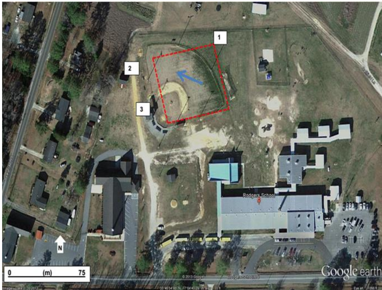
Figure 1. A permeable reactive barrier was installed between the septic drain field (red rectangle) and well 2. Well 2 had groundwater \text{NO}_3^- concentrations that routinely exceeded 10 mg/L.
