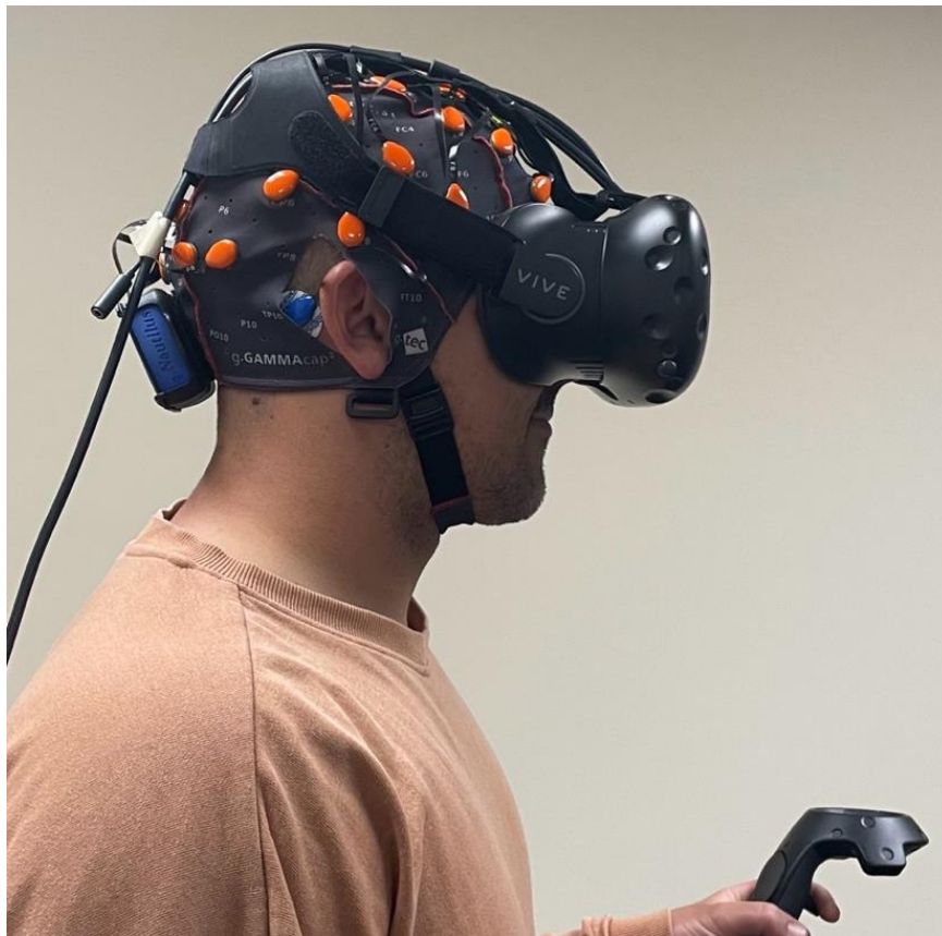
Figure 3: Participants were fitted with both an EEG cap as well as VR headset to complete a VR go/no-go task.
