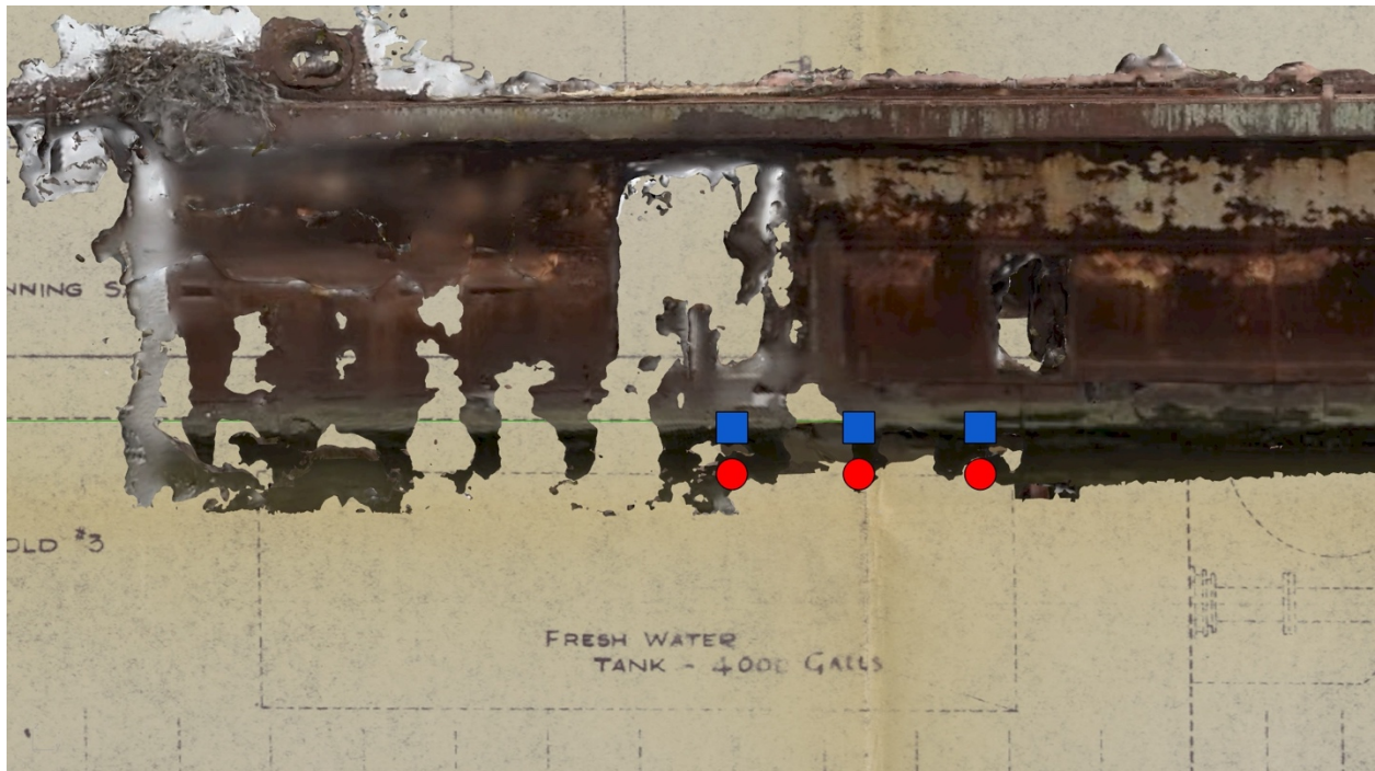
Figure 11. 3D model ( RhinoCAD-derived ) of starboard side (right) Accomac shipwreck overlaid onto blueprints showing bulkhead (back) biofilm samples. Blue squares represent biofilm samples taken at the water line and red circle samples represents biofilm samples taken below the waterline.
