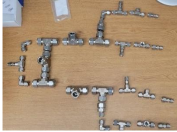
Figure 37: Metallic compression fittings laid out prior to assembly, connecting tubing is not shown.
