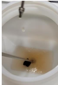
Figure 105: Rust colored water from corrosion caused by the NaCl brine
