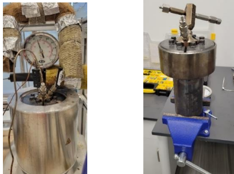
Figure 75: The Reactor (R1) in situ (Left), Reactor in vise for routine maintenance (Right)
