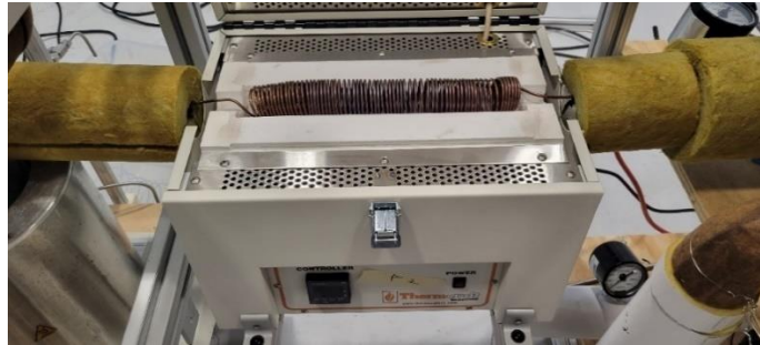
Figure 52: Furnace coil installed in Furnace 2
