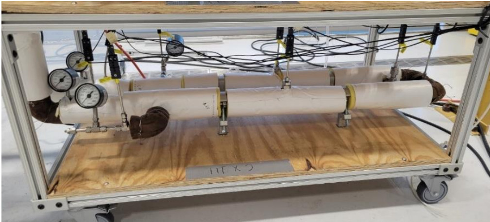
Figure 65: HEX2 wrapped in Fiberglass insulation.
