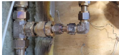
Figure 108: HEX1 hot line entrance and cooling line exit union
