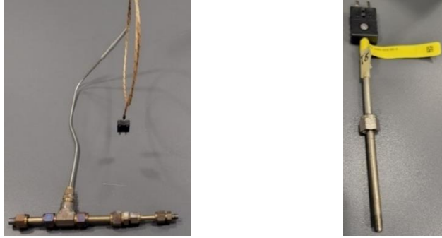
Figure 70: 1/8" X 12" Thermocouple that was used to measure the Reactor exit temperature (Left); 1/4" Diameter 6" long Thermocouple with metallic compression fitting (Right)
