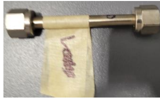
Figure 116: ¼” diameter thick-walled tubing with pin hole leak
