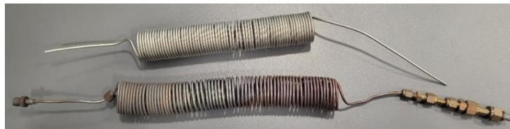
Figure 51: Furnace coil (top), Used furnace tube coil with fittings (Bottom)
