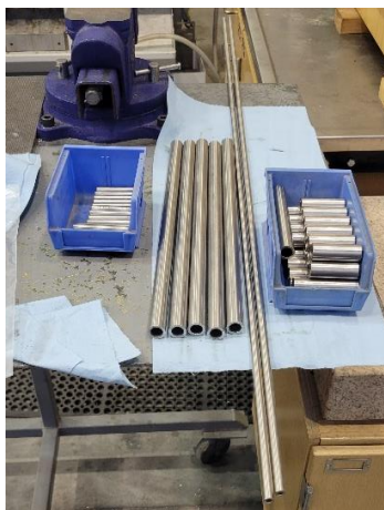
Figure 35: 316 Stainless-steel tubing prepared for fabrication
