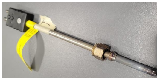
Figure 107: Thermocouple T1 from HEX1 after all experiments were completed.
