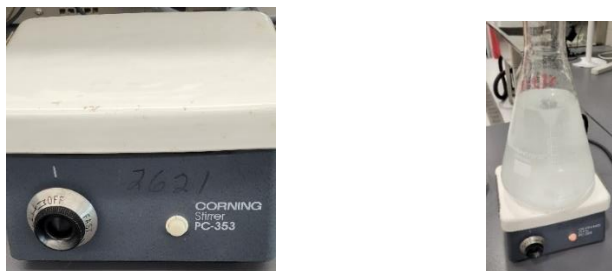
Figure 56: Corning PC-535 Stirrer alone (Left), Stirrer mixing 14wt% NaCl Brine (Right)
