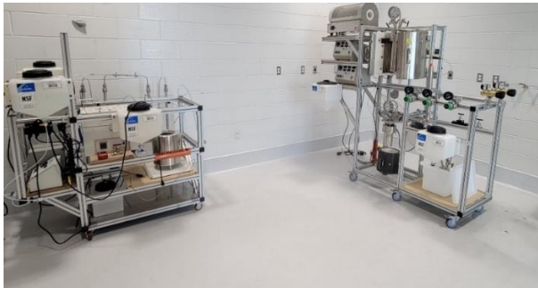
Figure 58: 10 ml/min Cart (Left), 10X 100 ml/min Desalination System (Right)
