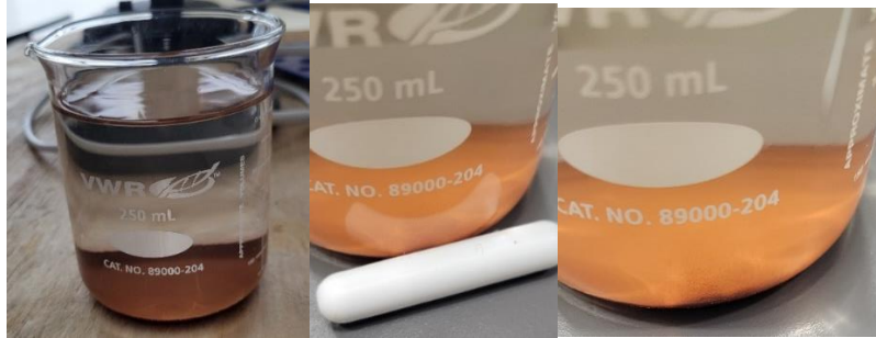
Figure 106: Rust mound at beaker wall caused by magnetic stirring bar
