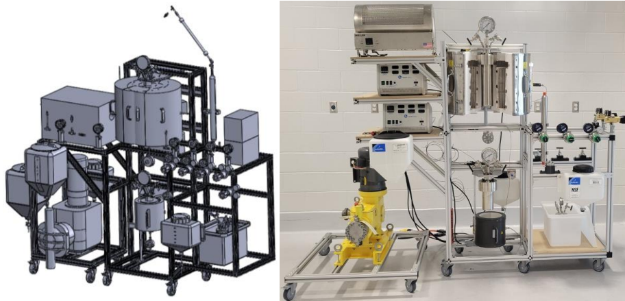
Figure 28: CAD Model (Left) and fabricated system 100mL/min desalination system also known as the 10X system (Right)
