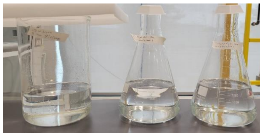
Figure 57: Finished mixed brine of 14wt%, 7.5wt% and 3.5wt% NaCl.
