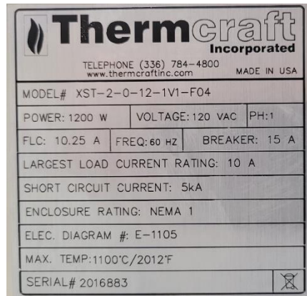
Figure 45: Furnace 1 and Furnace 2 Name plate data
