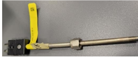
Figure 39: Thermocouple used on HEX2 at point T8 pulled for inspection.
