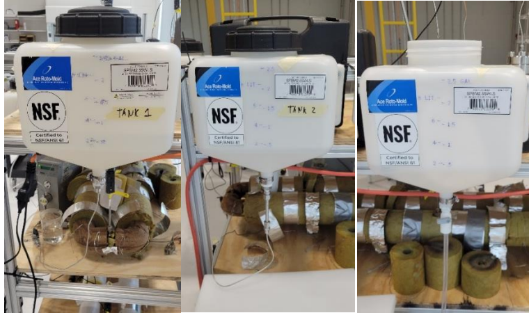
Figure 31: Tank 1 is for H 2 O, Tank 2 is for 3.5wt%, 7.5wt%, 14wt% NaCl Brine, HEX1 shell output tank
