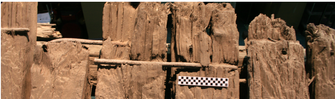
FIGURE IV.7. Jackson's drift fastening pattern (Photograph by author, 2009).
