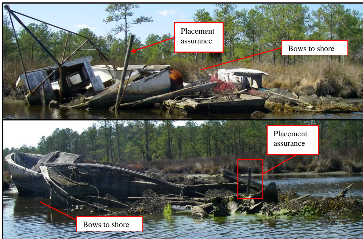
FIGURE 182. Vessels 8-10 and 39 (not visible) along west shoreline, grounded bow to shore, awash, and with placement assurance and some marine debris (top, facing southwest) (Marcotte 2008). Vessels 10-12 on adjacent east shoreline, grounded bow to shore, awash, with placement assurance and marine debris (bottom) (Marcotte 2008).
