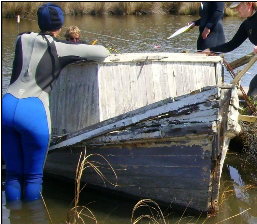
FIGURE 127. Vessel 10 with partially disarticulated starboard and port strakes, and forward wheelhouse (Marcotte 2008).
