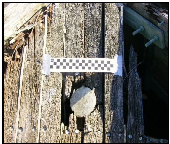
FIGURE 133. Vessel 12, detail of longitudinal bow planking and caulking (Latta 2008).
