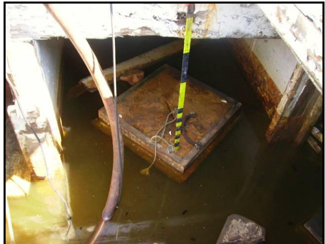
FIGURE 102. Flooded hold in Vessel 6. Note rubber pump hose running from bottom left (Latta 2008).
