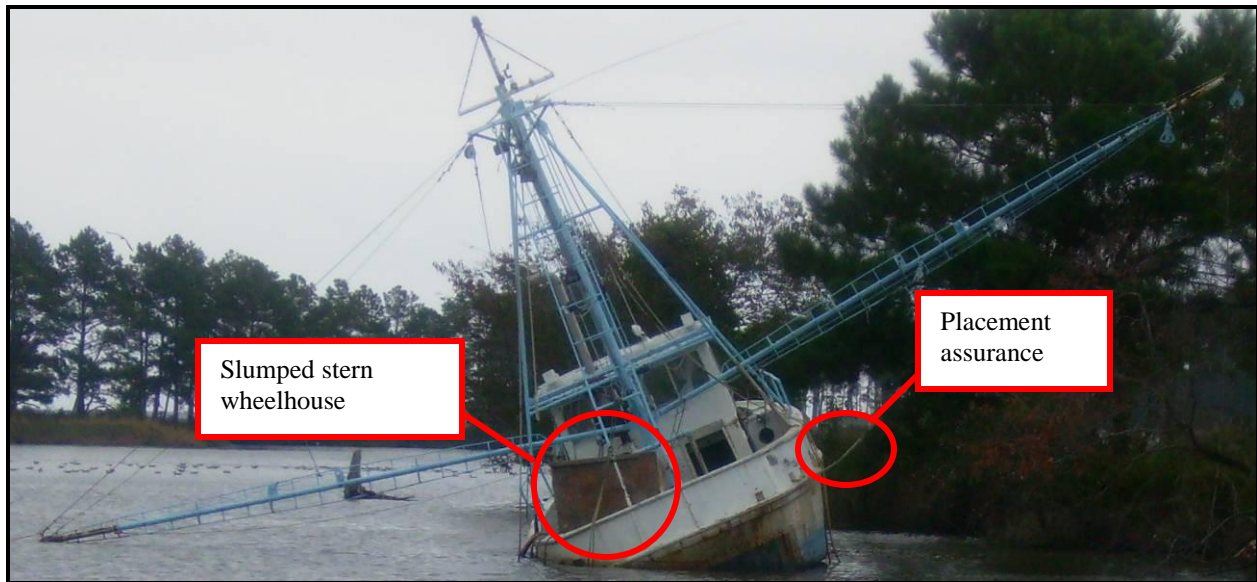
FIGURE 68. Vessel 31, Miss Alicia , with stern wheelhouse slumped to the port railing (Marcotte 2008).
