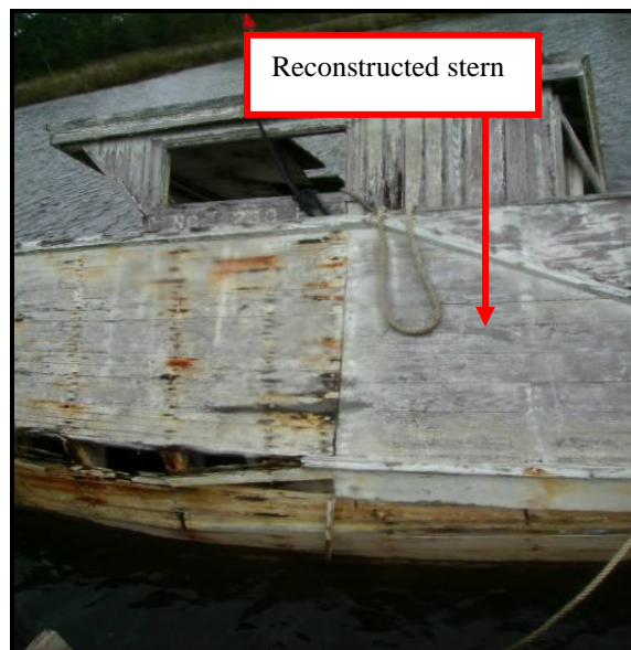
FIGURE 89. Vessel 19, port side bow deterioration and reconstructed stern. Salvage hole visible in roof (Marcotte 2008).
