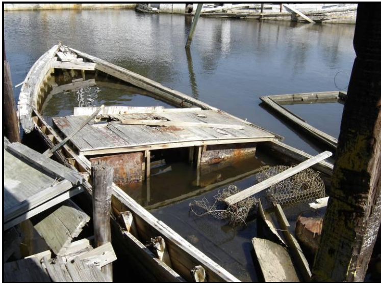
FIGURE 92. Vessel 3, evidence of salvage to upper wheelhouse and railing, and marine debris (Wagner 2008)
