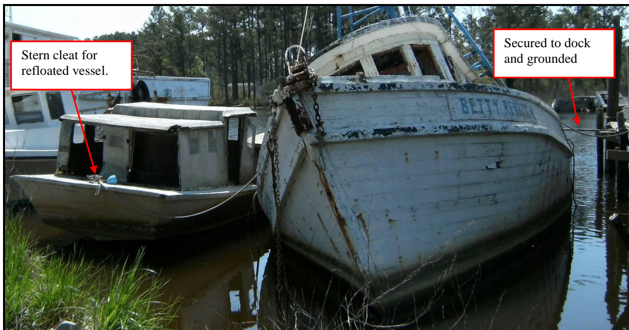
FIGURE 165. Placement assurance and orientation of Vessel 23 (left) and Vessel 24 (right), grounded and secured to dock and between vessels (Marcotte 2010).
