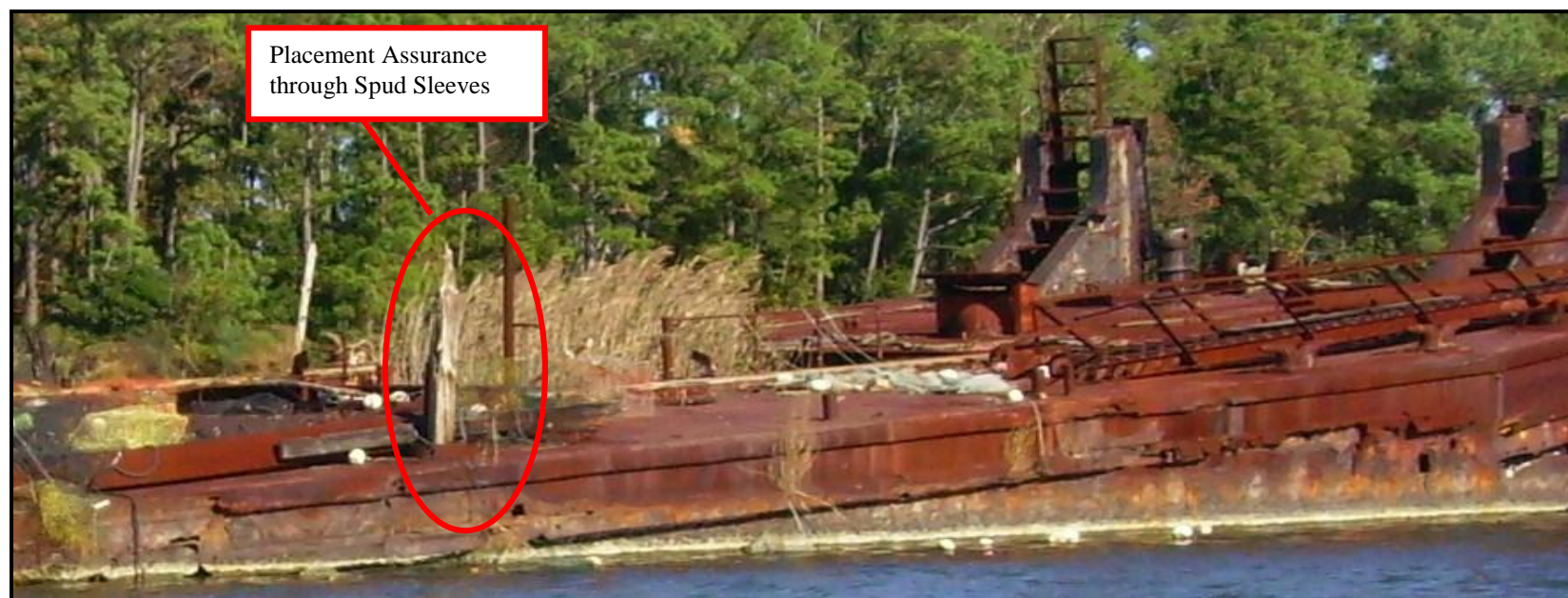
FIGURE 110. Vessel 13 ( Fred W. Olcott ), detail of placement assurance and deterioration (Marcotte 2007).
