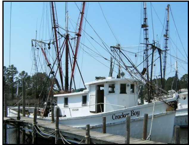
FIGURE 147. Cracker Boy after maintenance – marine paint and replacement of rub and cap rails (Marcotte 2010).
