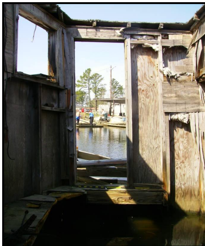
FIGURE 98. Vessel 5 ( Miss Amber ), showing detail of wheelhouse salvage and removal of roof (Marcotte 2008).
