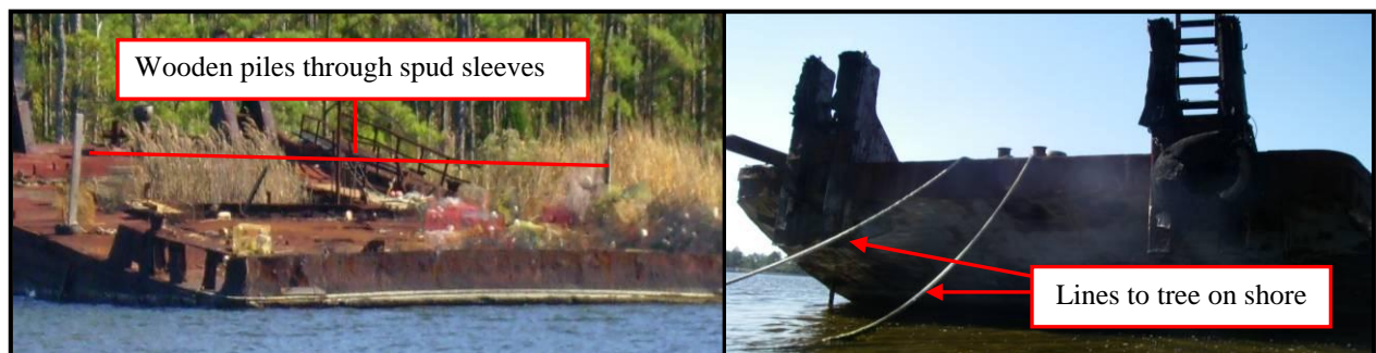
FIGURE 166. View of the stern of Vessel 13, highlighting spud sleeves (left, facing southeast) (Marcotte 2007). View of Vessel 13's bowlines (right, facing northwest) (Marcotte 2008).
