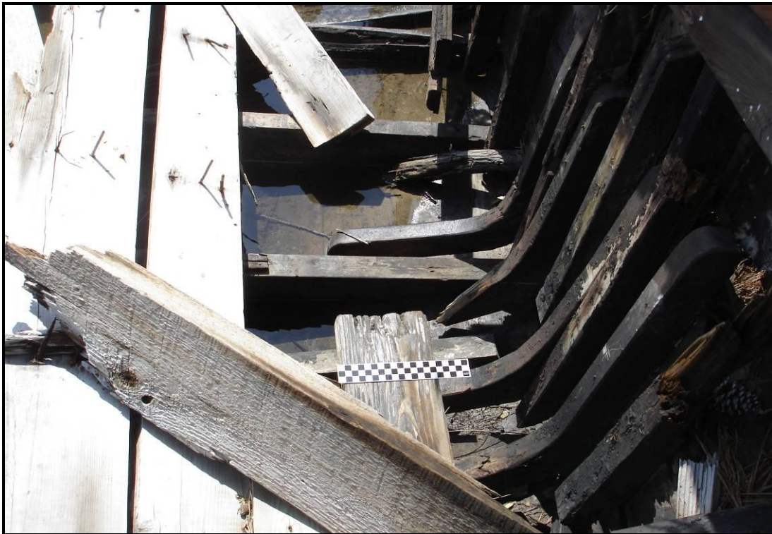
FIGURE 57. Vessel 1 ( Miss Shirley ), cypress compass timber scantlings (Ray 2008).
