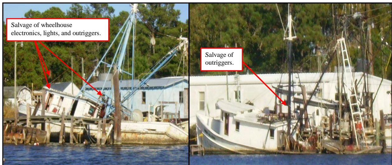
FIGURE 167. Vessel 22 ( Betty Rebecca ) left, and Vessel 24 ( Miss Allena ) right, both under partial salvage in November 2007 (Marcotte 2007). Note presence of fishing gear on stern of Vessel 24, as well as intact wheelhouse structure (Marcotte 2007).
