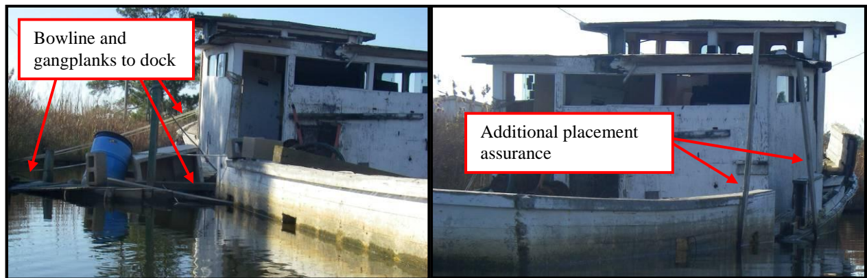
FIGURE 178. Vessel 15 showing construction of gangplanks (left) and placement assurance (right) for storage vessel (Marcotte 2010).
