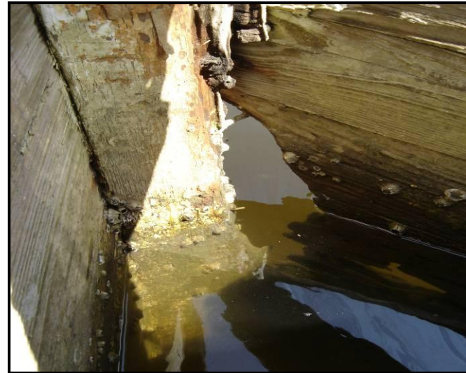
FIGURE 91. Vessel 3, detail of damage to bow near starboard side of stem (Wagner 2008).
