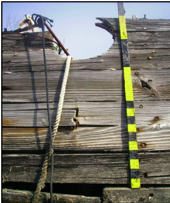
FIGURE 117. Vessel 7 - porthole, and pattern of fastening on strakes (Marcotte 2007).
