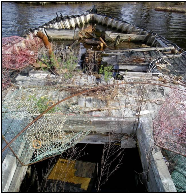
FIGURE 71. Fire damage to bow of Vessel 2 and remaining footprint of superstructure (Steinmetz 2008).
