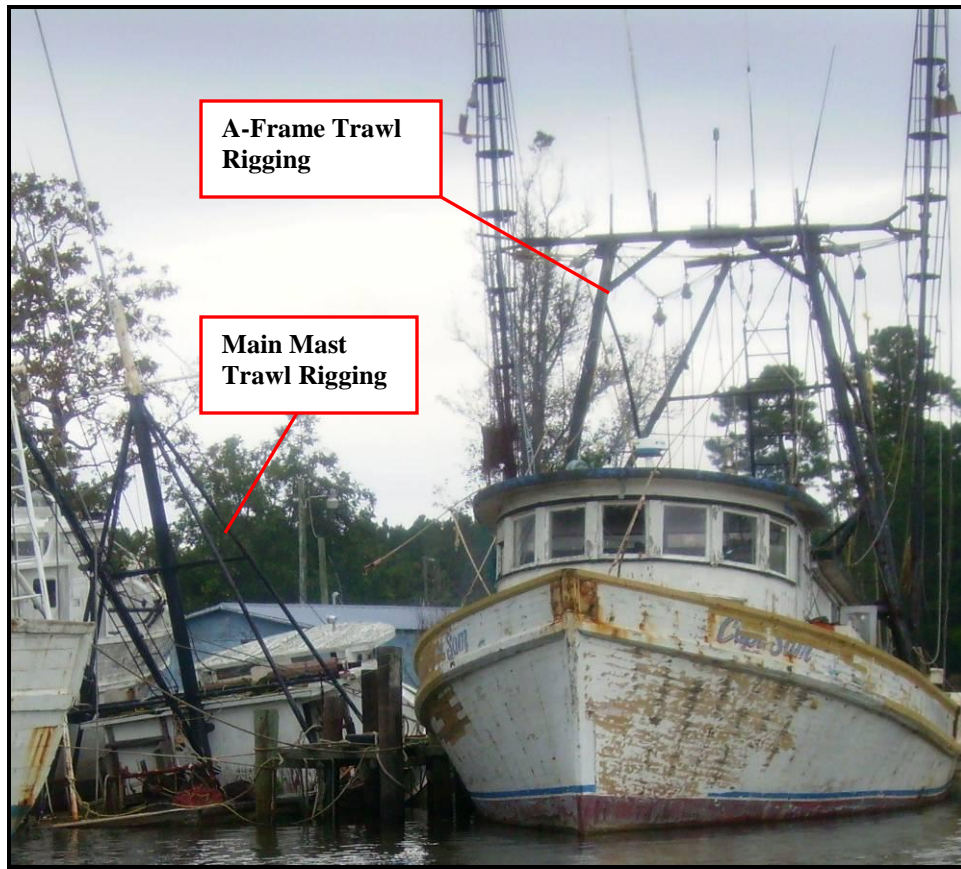
FIGURE 142. Foster's Seafood Complex vessels displaying both main mast rigging and A-frame rigging (Marcotte 2008).
