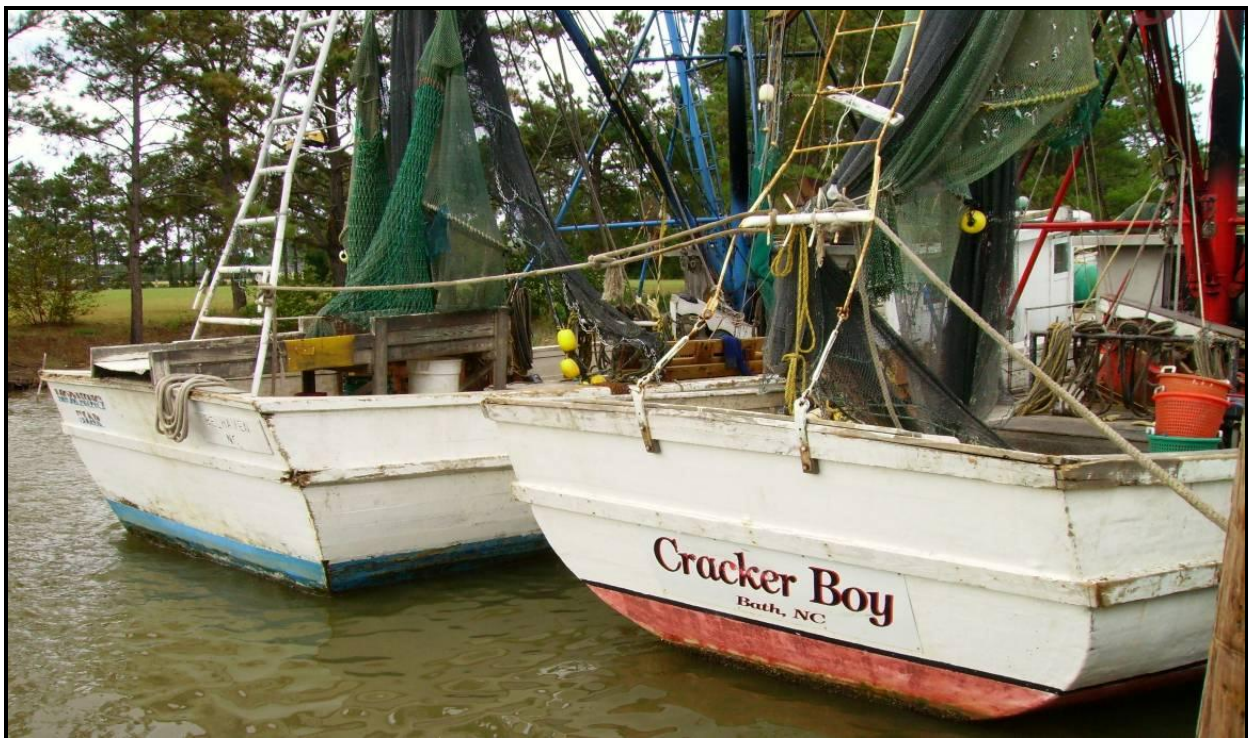
FIGURE 144. Comparison chine bottom vessel ( Morning Star , left) and vessel constructed of steamed, curved ribs ( Cracker Boy , right) (Marcotte 2008).
