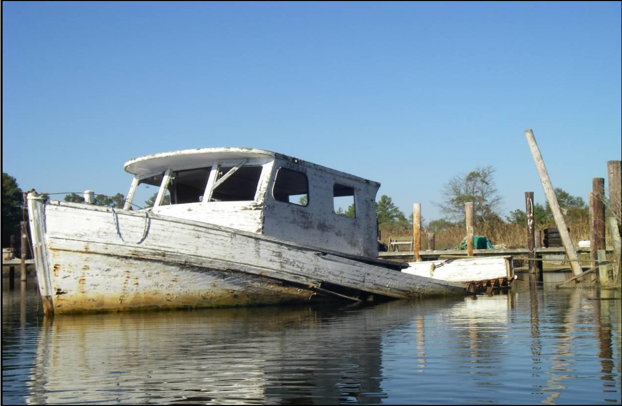
FIGURE 84. Vessel 16, after salvage of trawl rig on stern end, and deteriorated port side (Marcotte 2009).
