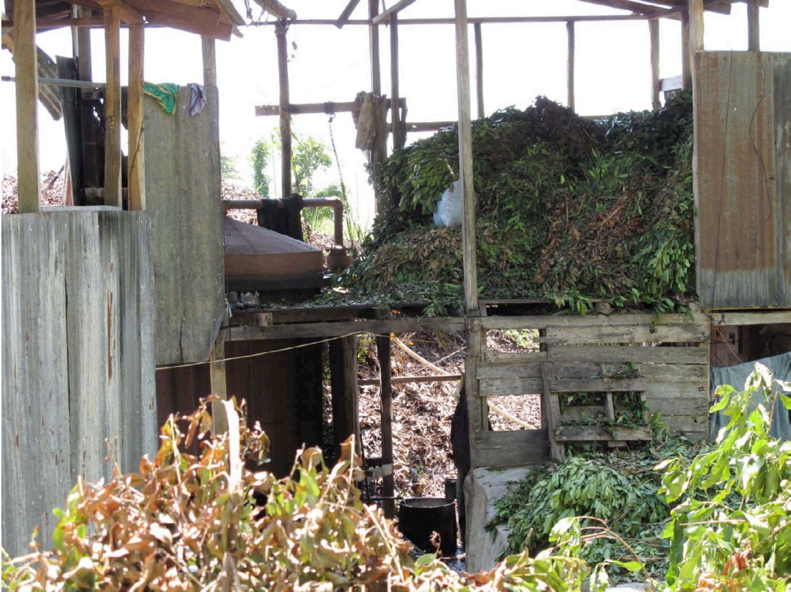
FIGURE 91. The Pimento Factory. Note the cast iron boiler on the left , the bushels of pimento leaves on the right , and the cooling barrel at the bottom . (Photo by author, October 13, 2009.)
