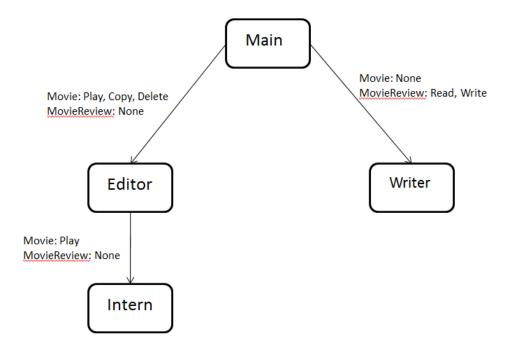
Figure 4: Model of the Example Network.
