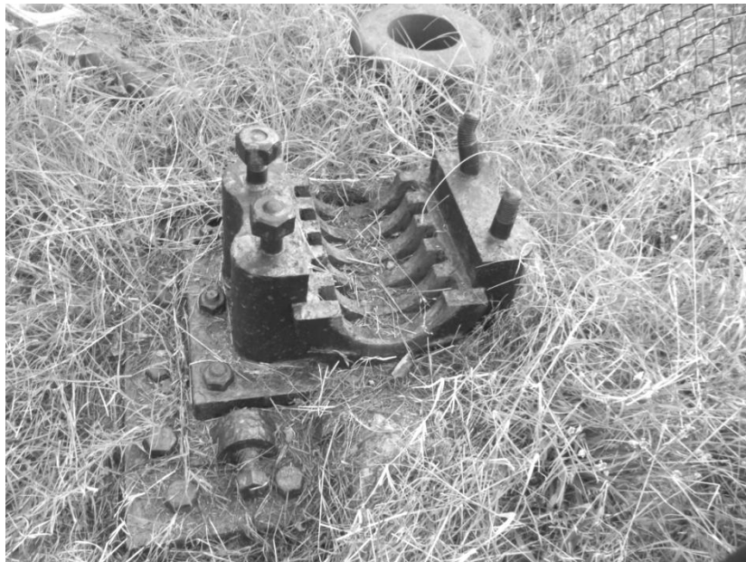
FIGURE VI.65. Large cast iron thrust bearing mounting block from either Jackson or Chattahoochee . (Photo by author 2011)
