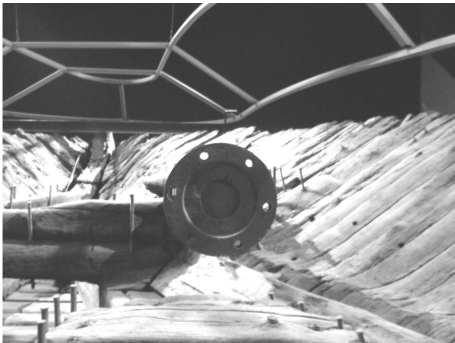
FIGURE VI.58. Jackson 's twin 7.5-foot diameter iron propellers and the sections of the shafts where they pass through the hull are preserved on the wreck today. (Photo by author 2011)
