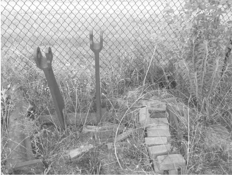
FIGURE VI.67. More parts of reversing gear assembly. The bricks at right were initially thought to be boiler bed firebricks but are not from either vessel. (Photo by author 2011)
