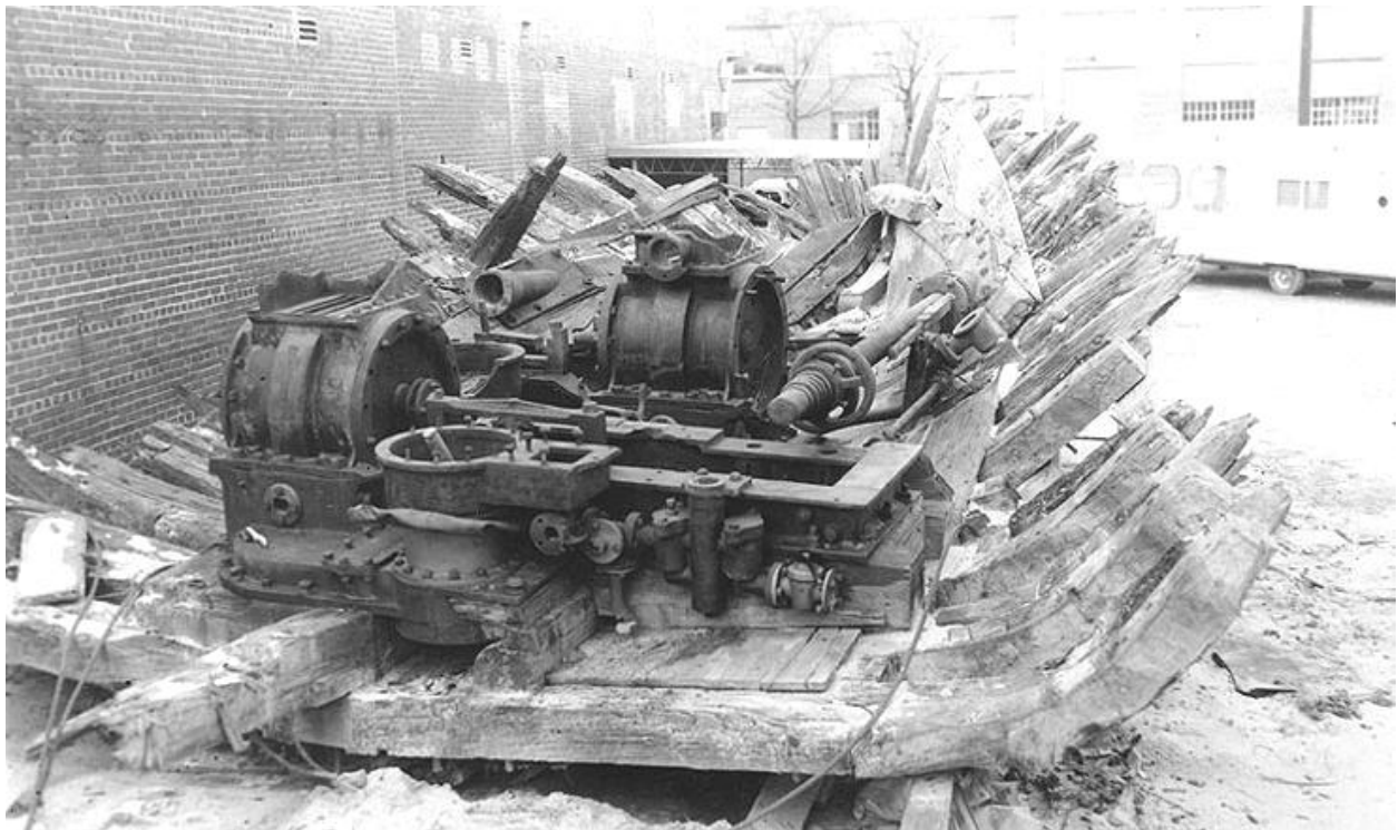
FIGURE III.14. The two horizontal direct-acting engines of CSS Chattahoochee . Each engine turned one screw on the opposite side of the hull from the cylinder head. (Online Library of Selected Images, Naval Historical Center, Department of the Navy, Washington, DC, 2012)
