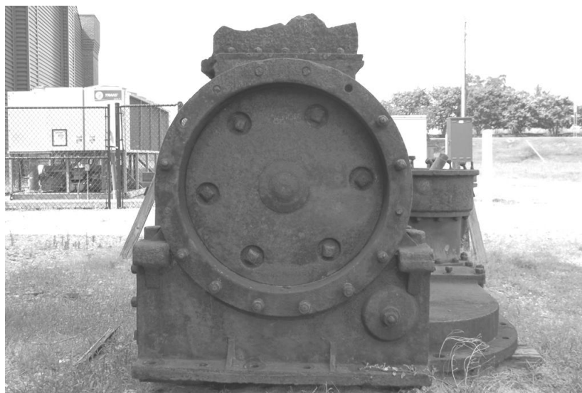
FIGURE VI.60. Front of the starboard engine. The cylinder head has been removed, showing the 28-inch diameter piston. (Photo by author 2011)
