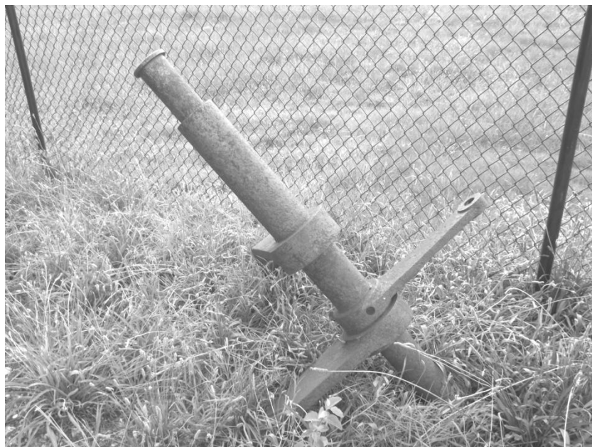
FIGURE VI.66. Part of reversing gear assembly for either Jackson or Chattahoochee . (Photo by author 2011)
