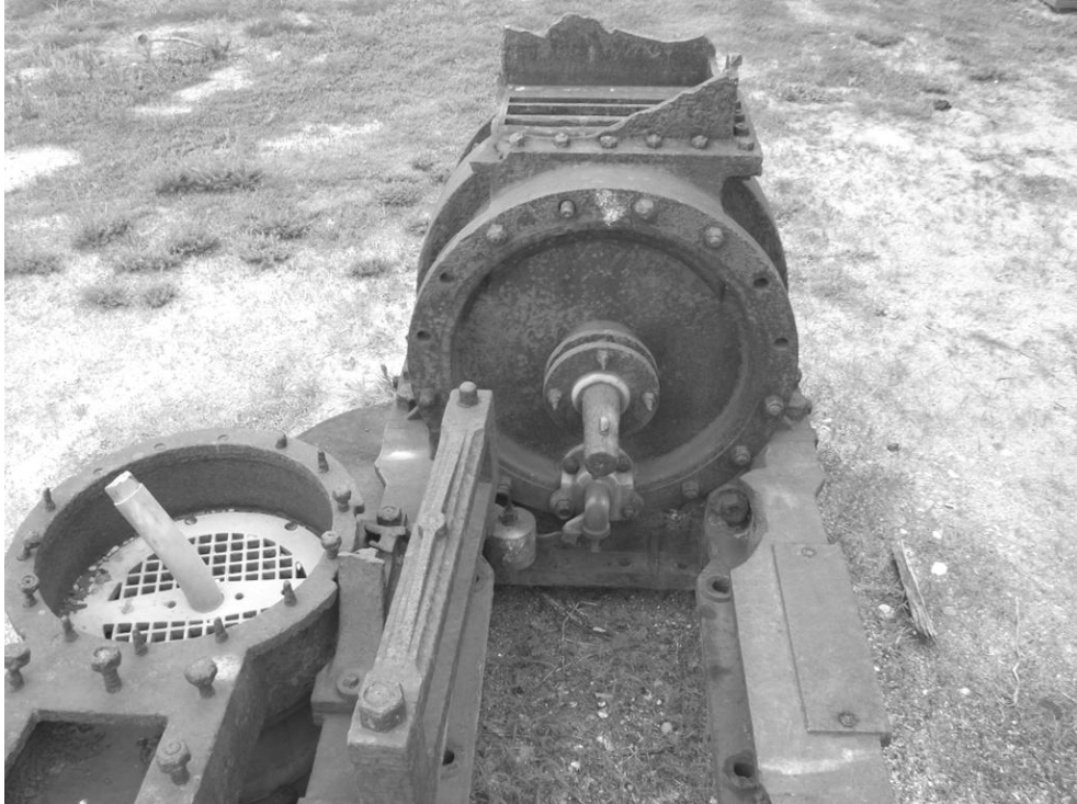
FIGURE VI.61. Chattahoochee 's starboard engine seen from above. The condenser, left, part of the crosshead guides for the connecting rod, and piston rod can be clearly seen. (Photo by author 2011)
