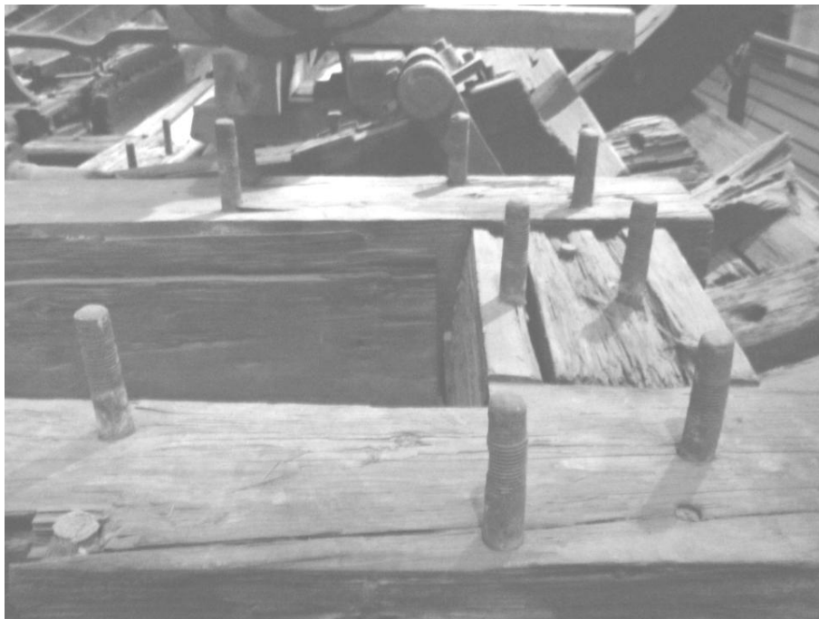
FIGURE VI.64. Engine mounting timberwork for the starboard engine in the preserved stern section of Chattahoochee . The timbers measure 9 inches sided by 12 inches molded on average, and the bolts measure 1.25 inches in diameter. Part of the port propeller shaft connecting assembly can be seen at the top of the image. (Photo by author 2011)
