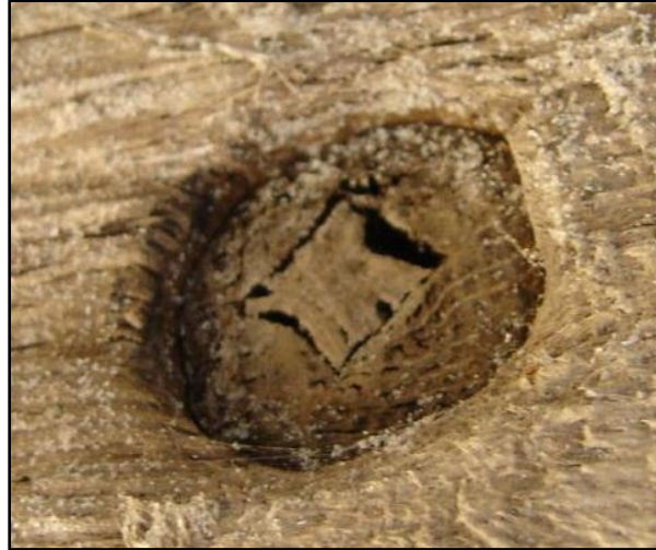
FIGURE 119. Square-pegged treenail from a hull plank on CKB0022. (Photo by Bradley Rodgers, 2010)
