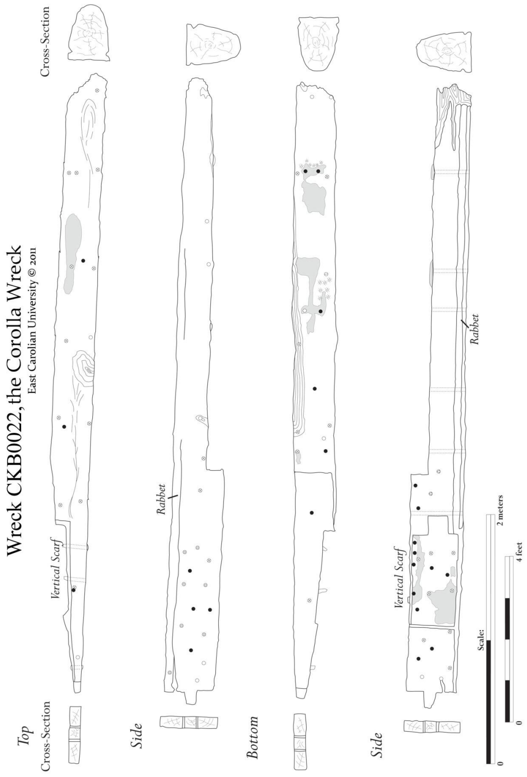
FIGURE 129. Keel recording of Wreck CKB0022. (© East Carolina University 2010)
