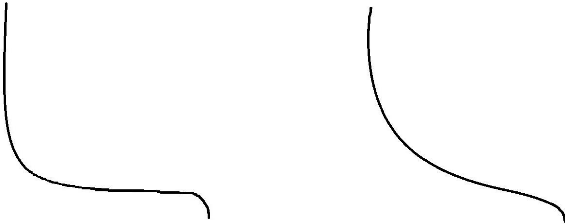
FIGURE 38. A flatter, bottom-based hull shape ( left ) compared to a curvier, frame-based hull shape ( right ). (By author 2013)
