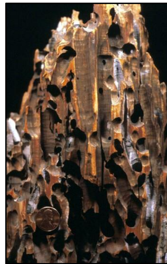
FIGURE 79. Shipworm ( Teredinidae ), also teredo worm, has caused damage to wooden vessels and submerged wooden structures for thousands of years. (Courtesy of Audubon.org, 2013) FIGURE 80. Teredo worm borings in a modern wharf piling. (Photo by Mark Wilson, 2008)
