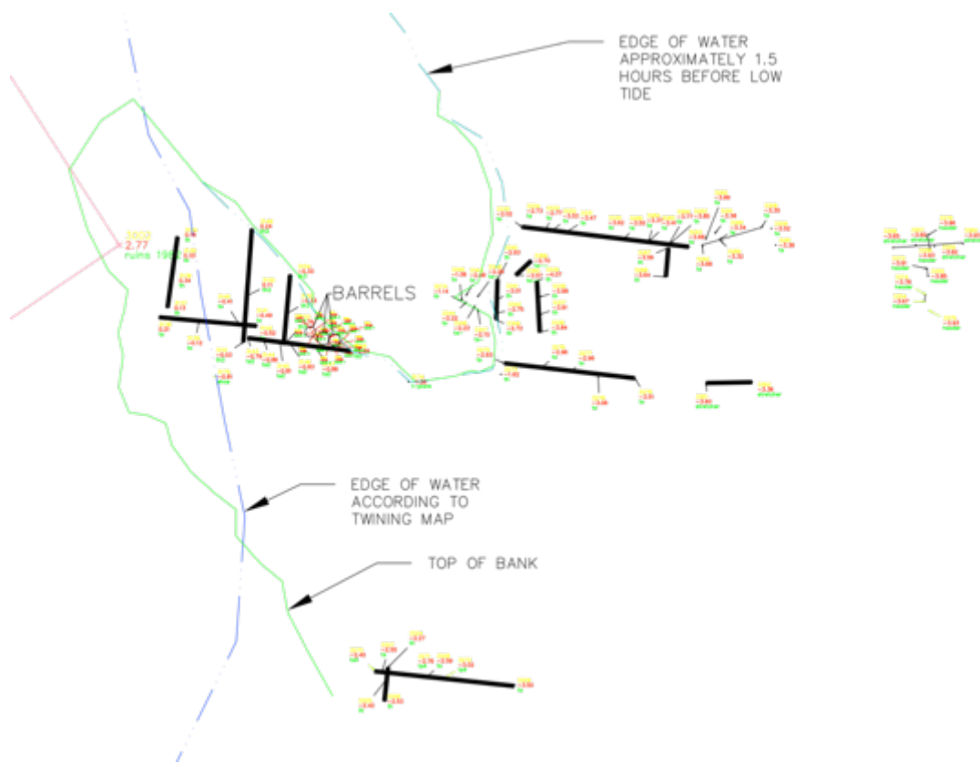
Figure 4. Map of Dry's Wharf based on survey data. Courtesy of Paul R. Shivers P.E. and David M. Edward P.L.S.
