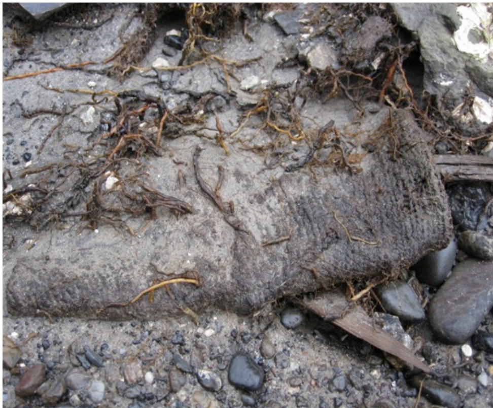
Figure 12. Brunswick Cap before recovery. The cap is just barely visible across the middle third of the photograph. The edge of the fold is just above the rocks in the bottom right corner.
