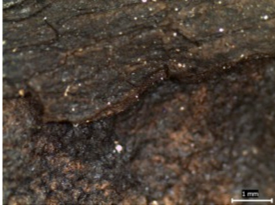
Figure 36. Grain side of Shoe #2 Note the cracking and delamination.
