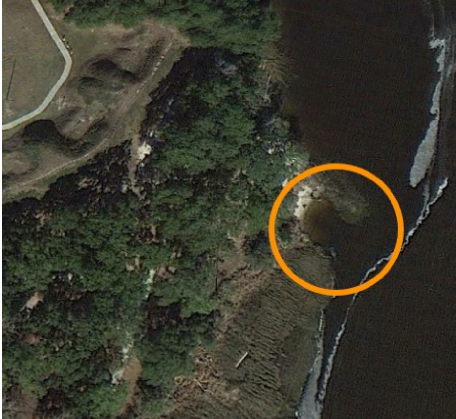
Figure 3. A 2013 Google Earth image of part of the BT/FA waterfront. The highlighted area indicates where the cut in the bank formed, and has expanded since the end of the 2000s.
