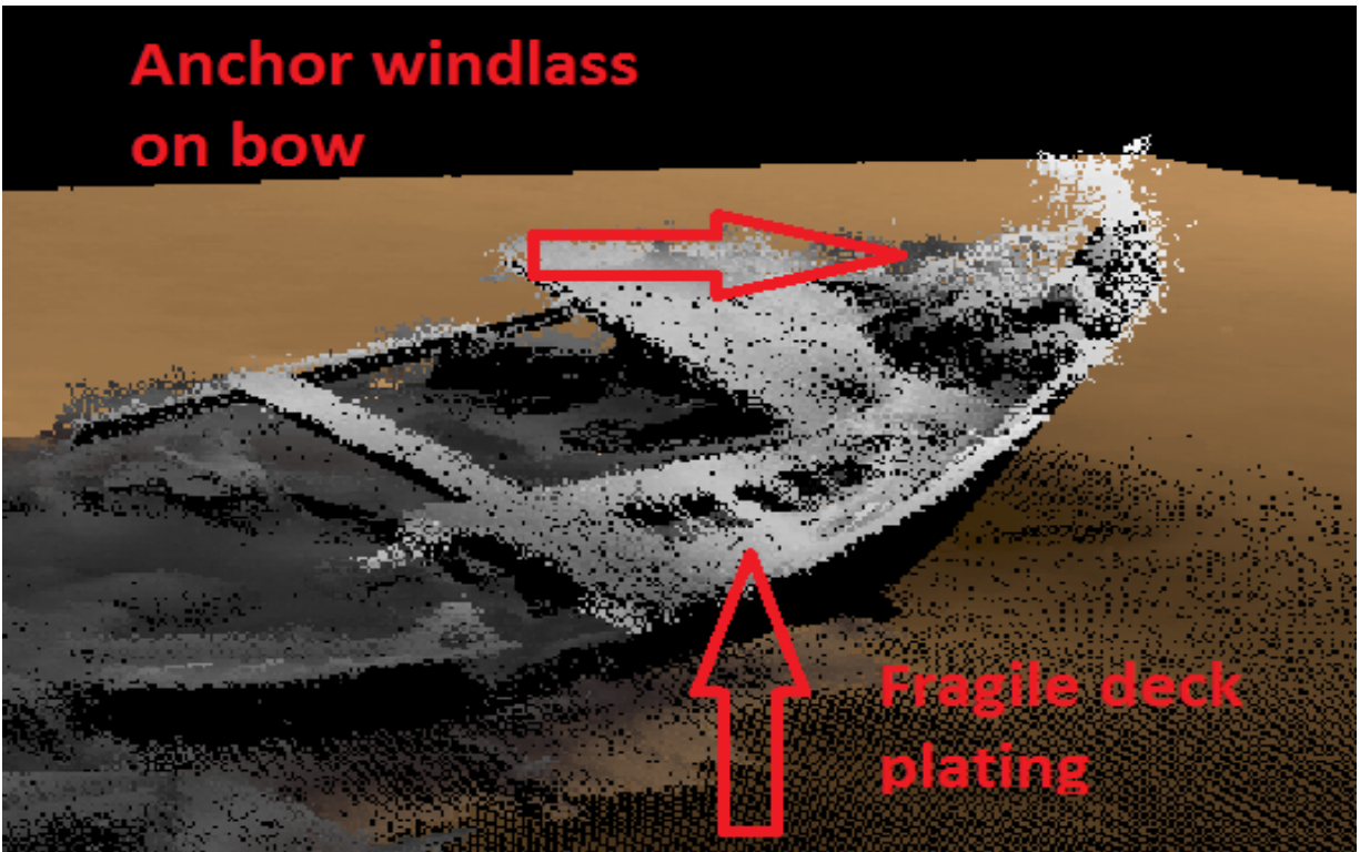
FIGURE 6.36. Multibeam image illustrating existing upper decking in bow stern (Source: NOAA).
