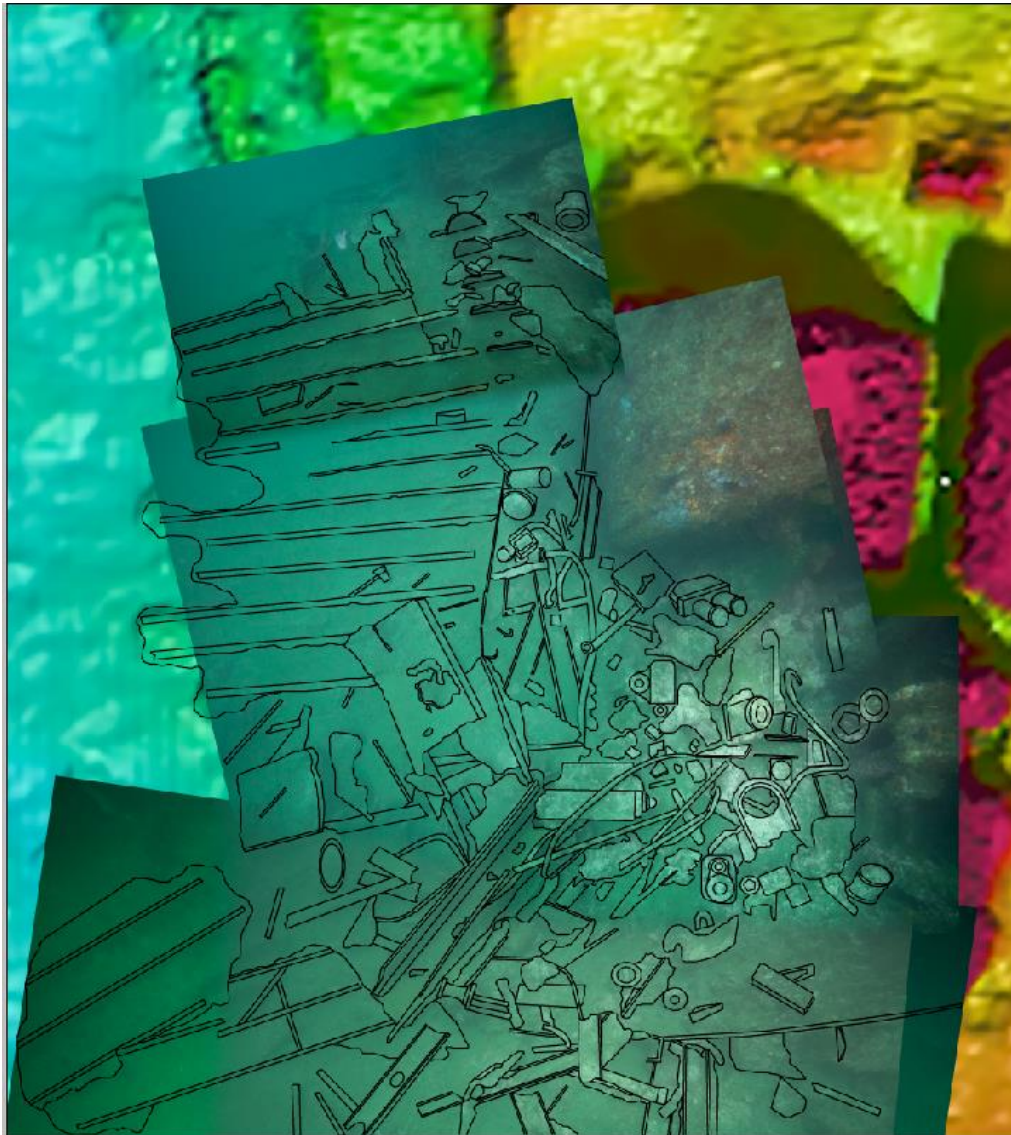
FIGURE 4.15. Example of the hybrid mapping technique using remote sensing imagery and scaled photographs in Adobe Photoshop (Image by Kara Fox).
