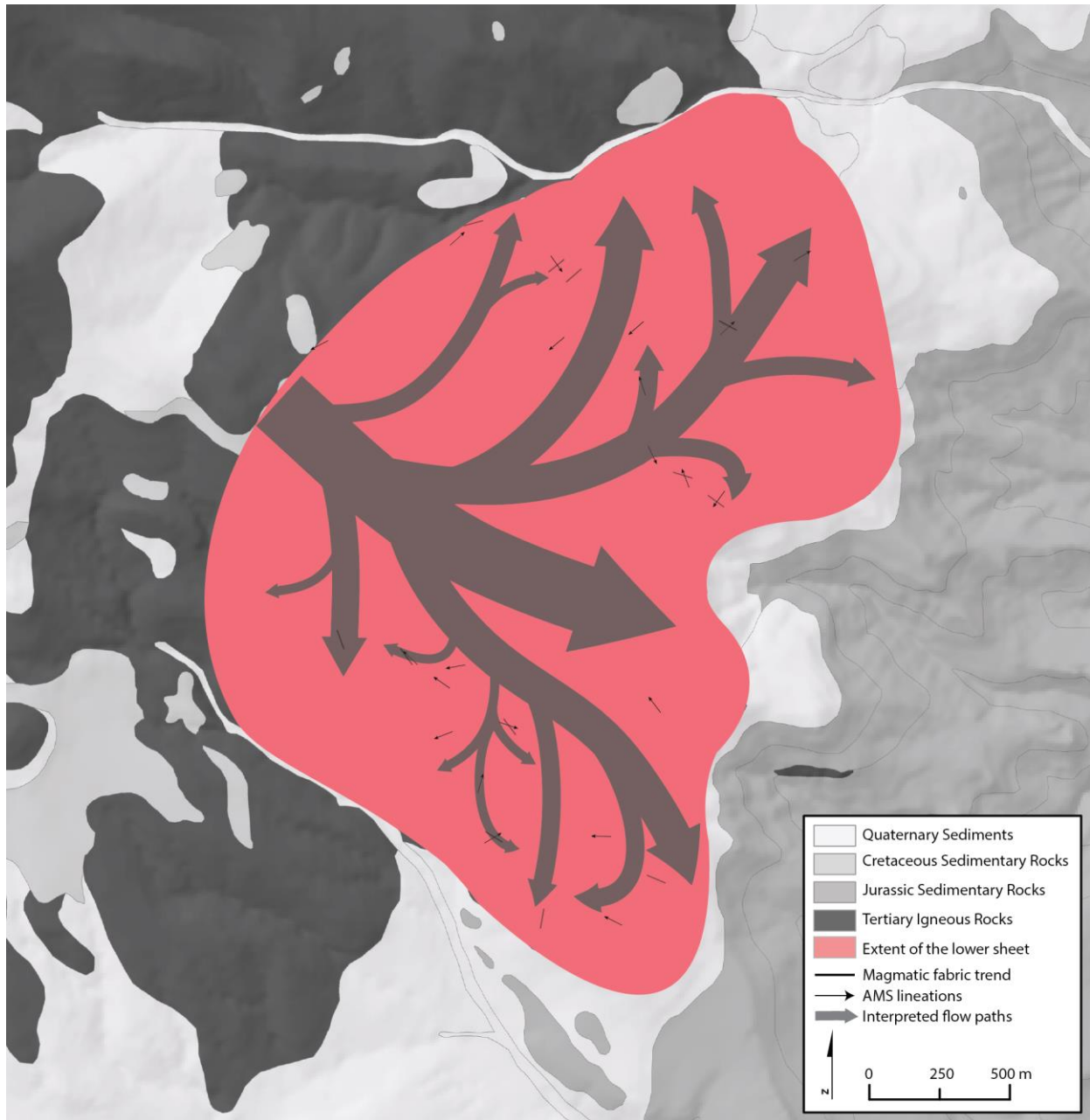
Figure 45. Interpreted flow paths during magma intrusion and formation of the lower sheet. Thin black lines with arrowheads indicate AMS lineations, and plain thin black lines indicate field fabric measurements.
