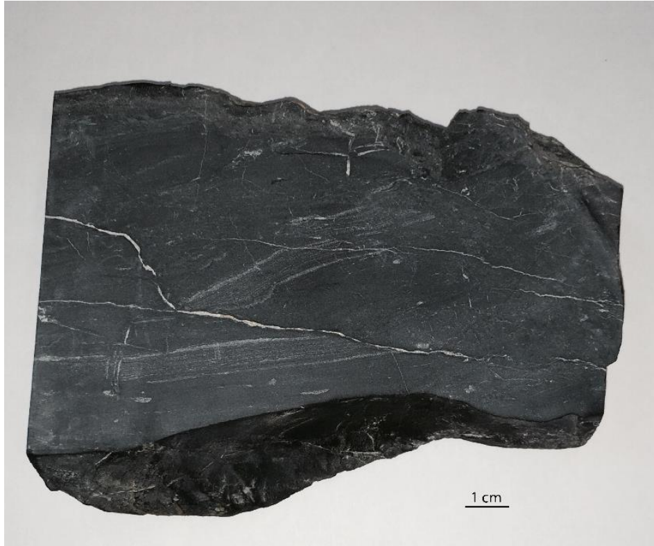
Figure 24. Image of metamorphosed Tununk sample, showing small-scale faults and calcite mineralized fractures.
