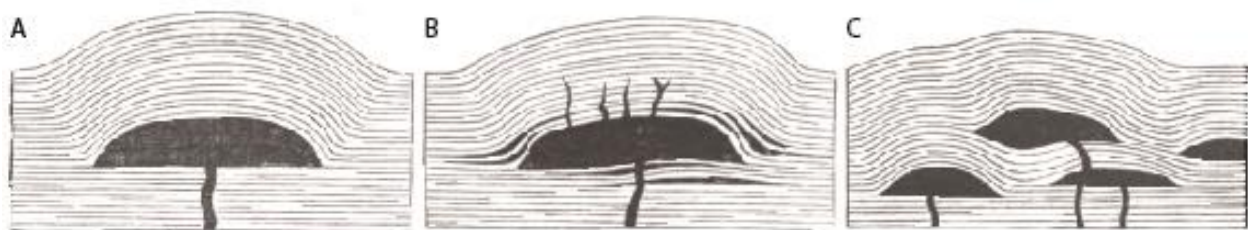
Figure 6. Sketches of idealized laccolithic intrusions (from Gilbert, 1877): A: Simple idealized laccolith. B: Laccolith with associated dikes and sills. C: Stacked laccoliths showing deformation of the overlying strata.
