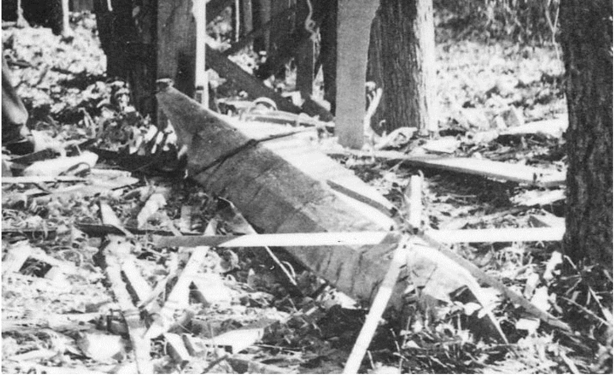
FIGURE 34. Detail of upside down bottom piece in Creef boatshop photo (Photo Courtesy of the Smithsonian).
