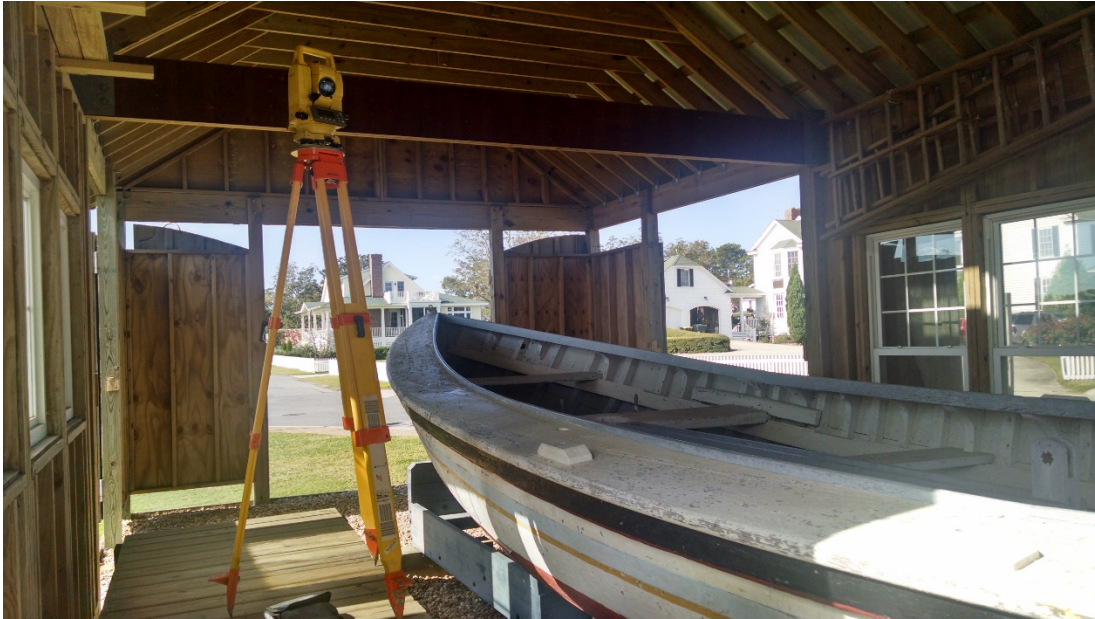
FIGURE 22. Total station setup for recording timber locations in hull. Location is the far right point in Figure 21 (Image by Author).
