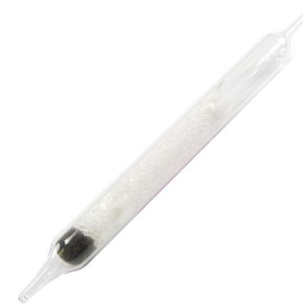
Figure 3. Silica gel tube as sampling media (Source: www.skinc.com/ )
