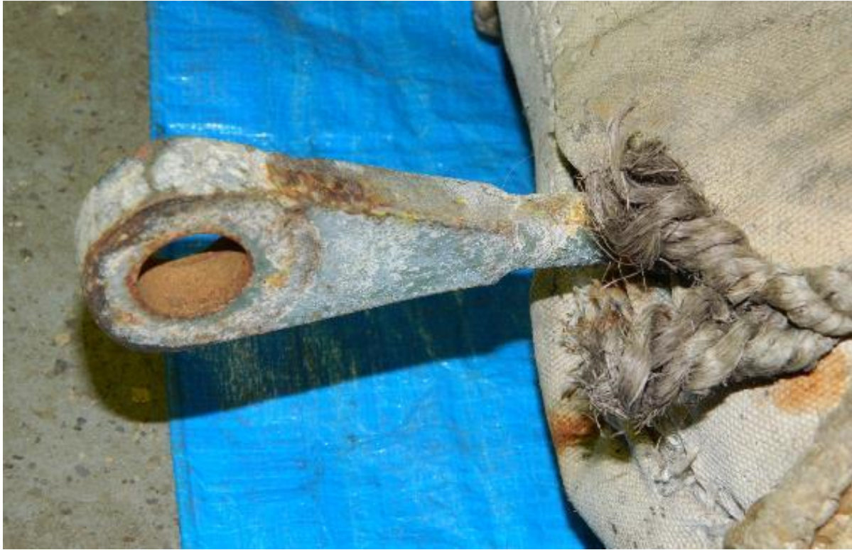
FIGURE 32. Metal eye on the sea sled's support beam for attachment of a cable to the ship's crane (Author 2013)
