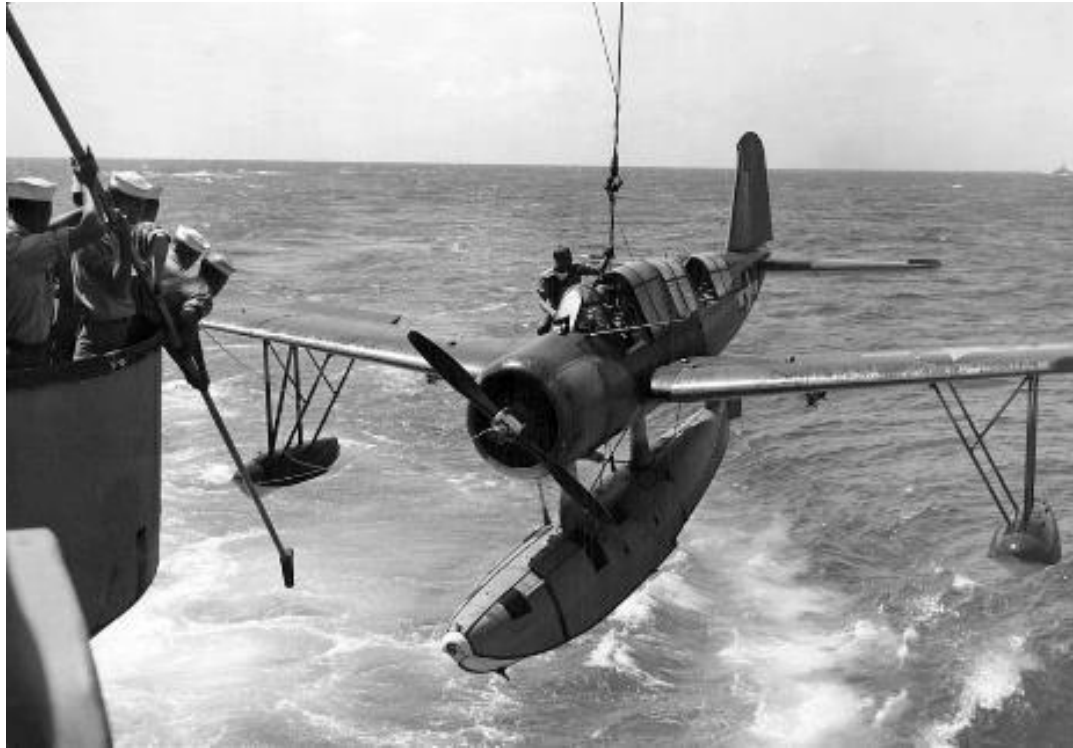
FIGURE 21. Kingfisher attached to sea sled and being lifted by crane (Darling 2001: 57)
