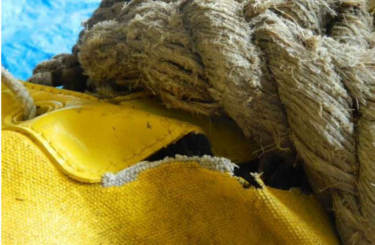
FIGURE 27. The lacing has caused the sack to come apart (Author 2013)
