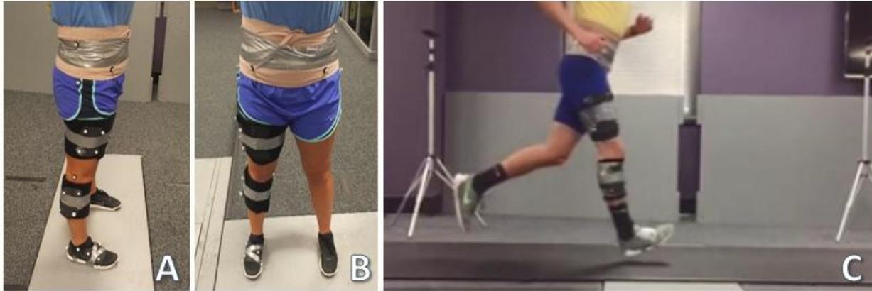
*Figure 9: Marker and EMG placement from the sagittal (A) and frontal (B) plane. Visual representation of the protocol setup with participant running across condition 2 (C).*
