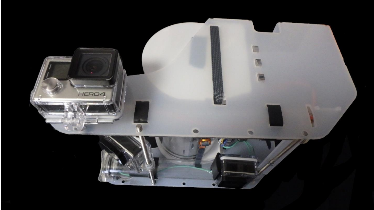
Figure 3. OpenROV 2.8 outfitted to capture profile view (K. Clevenger 2016).
