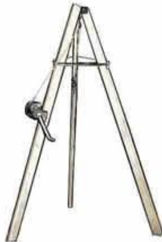
Figure 1. Tripod apparatus used in weighing shaded and exposed subjects
