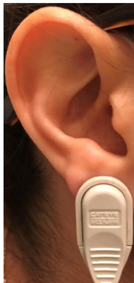
Figure 4. Ear lobe sensor positioning for optical pulse measurements
