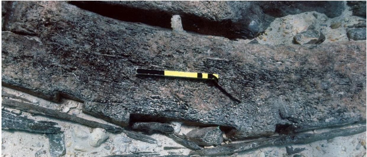
FIGURE 5.10. Keel step in T1, scale bar is 15 in. (38 cm). (Image from NPS, 2016).
