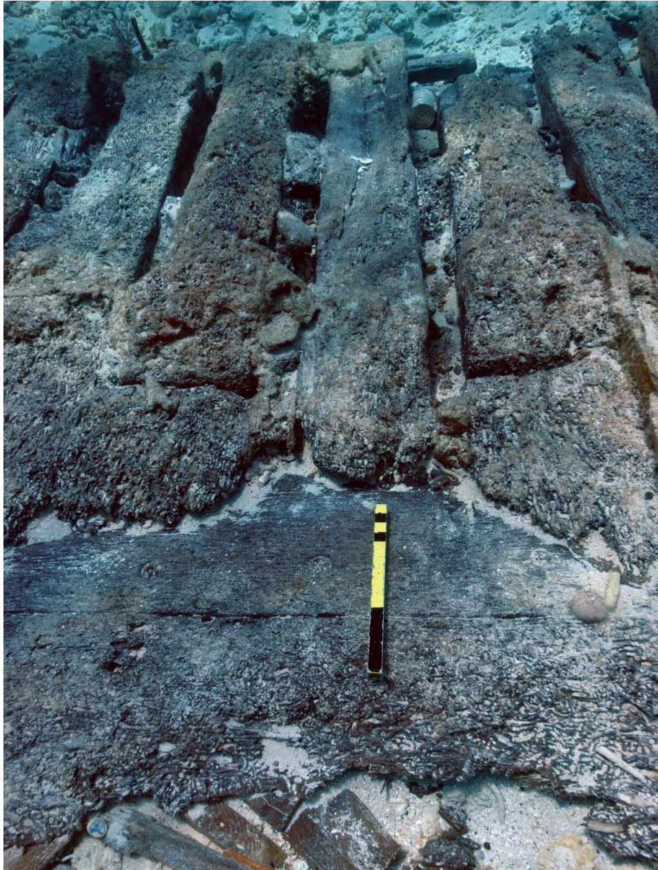
FIGURE 5.6. Additional futtocks (T48 and T49) with squared butt joints. Scale is 15 in. (38 cm) and in line with T39. (Image from NPS, 2016).
