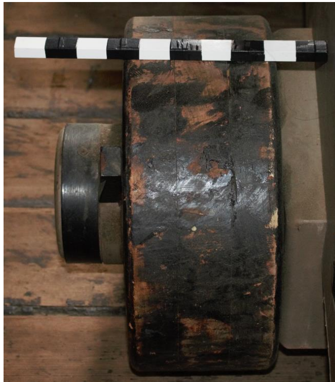
FIGURE 4.21: Rear Axletree arm and truck for Carriage 17, U.S.S. Constellation . Photograph taken by author in 2018.
