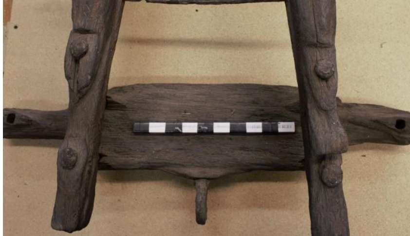
FIGURE 3.29: Rear ring bolt for Royal Savage carriage, at Fort Ticonderoga. Photograph taken by author in May 2018.
