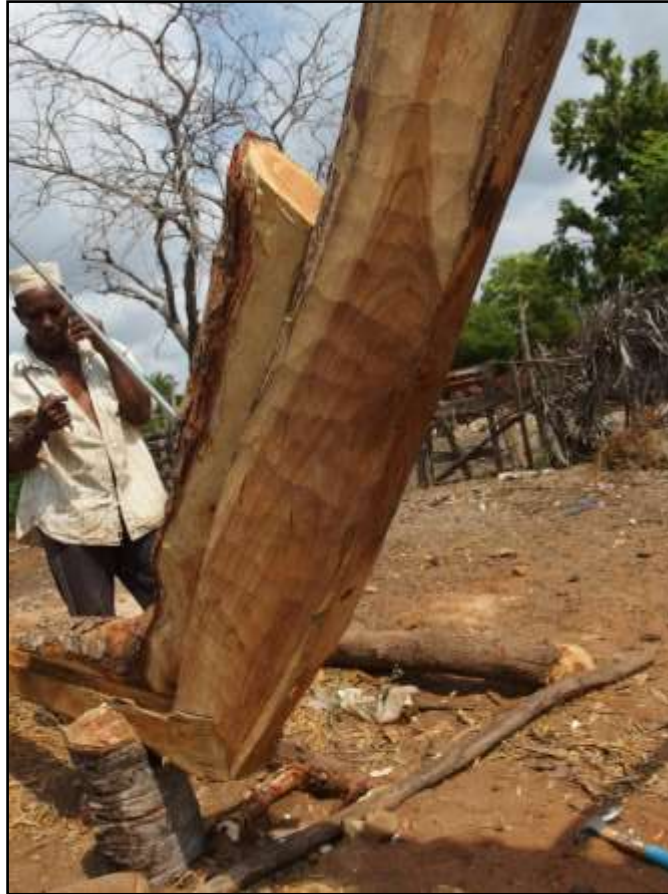
Figure 27: Mfundu Muddi secures the lag bolts of the sternpost on a large ocean-going dau , Tongoni Village, Tanga Region (Photograph by Madeline Roth)
