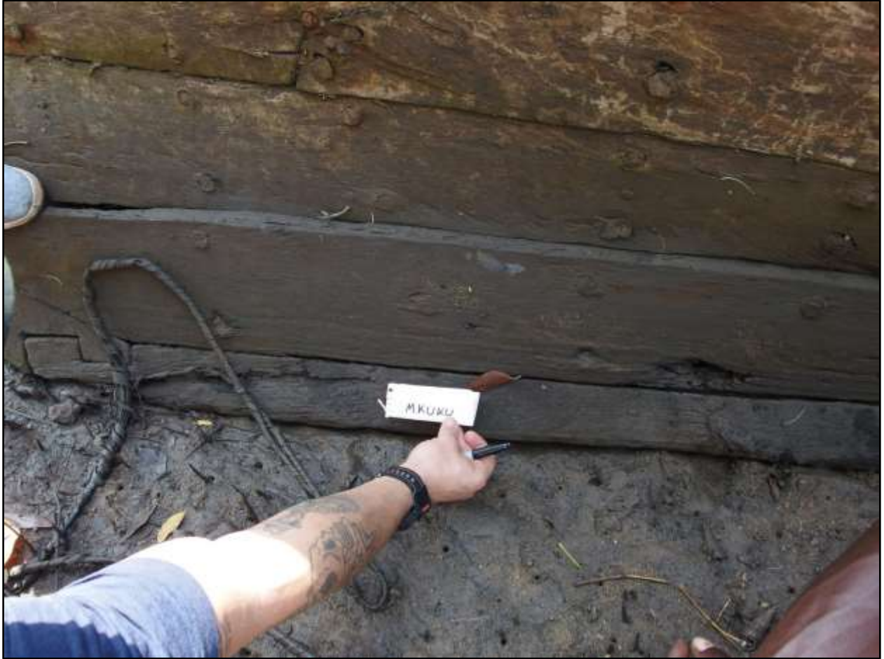
Author indicating the mkuku , or keel, Tongoni Village, Tanga Region (Photograph by Madeline Roth)
