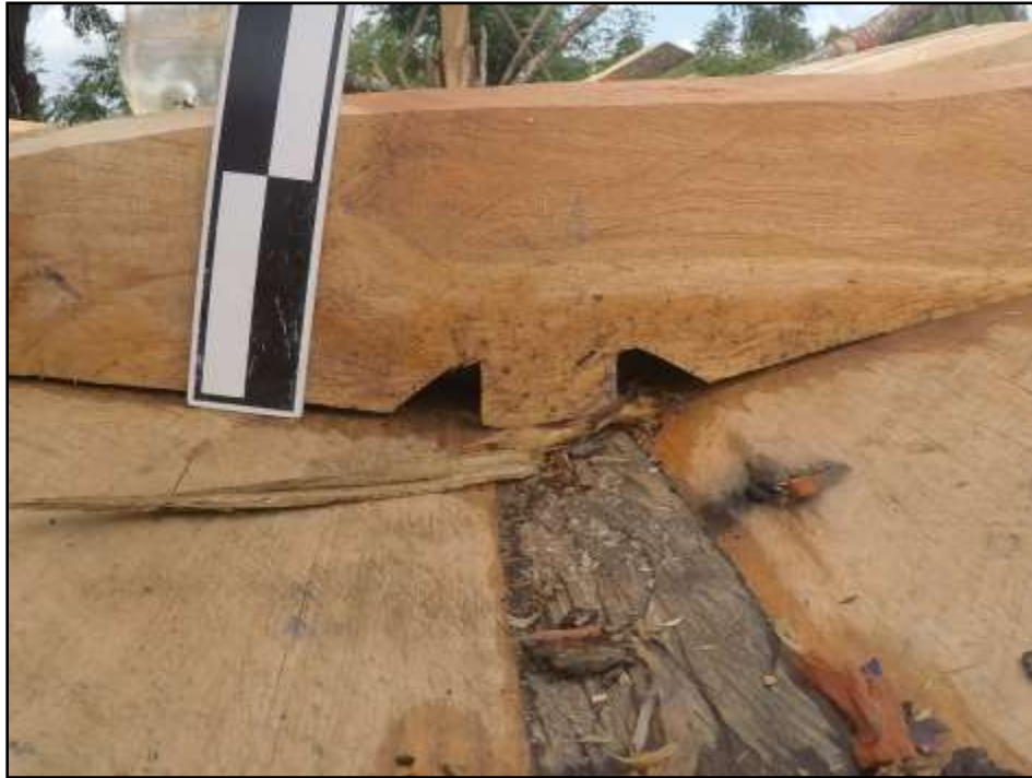
Figure 28: Scaled photograph of the njia ya maji , or waterway, seen on all Y-frames emplaced along the keel of the dau , Tongoni Village, Tanga Region (Photograph by author)
