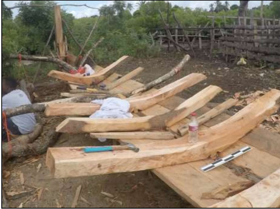
Figure 29: Dau with emplaced Y-frames, garboard strakes, and stern post with weighted arms for plank forming visible, Tongoni Village, Tanga Region (Photograph by author)
