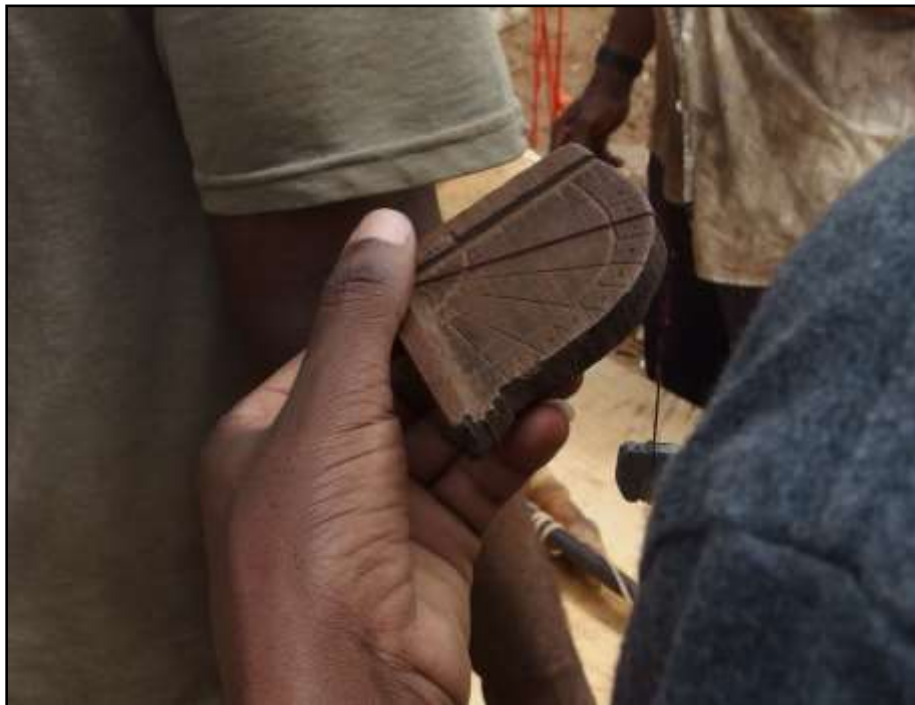
Figure 21: Mfundu Muddi demonstrating the use of the handi to interpret to check Y-frame angle, Tongoni Village, Tanga Region (Photograph by Madeline Roth)
