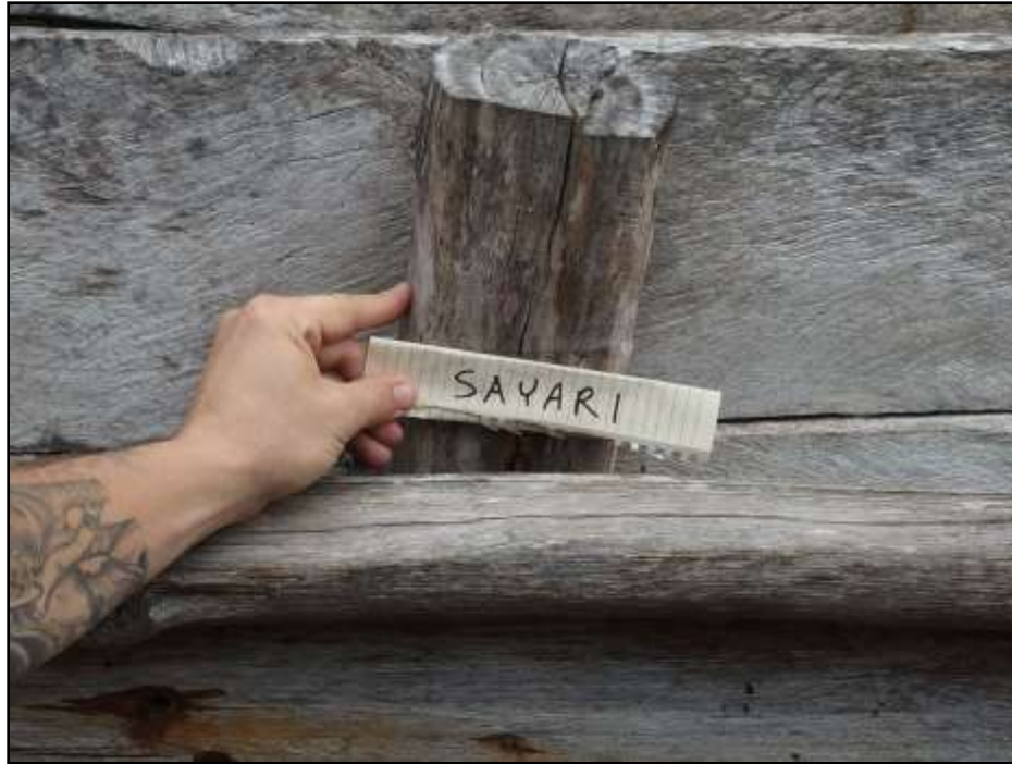
Figure 19: KiSwahili nomenclature for framing element named sayari (planet) within a discarded sampa (flat-bottomed dau ) vessel, Tongoni Village, Tanga Region (Photograph by Madeline Roth)
