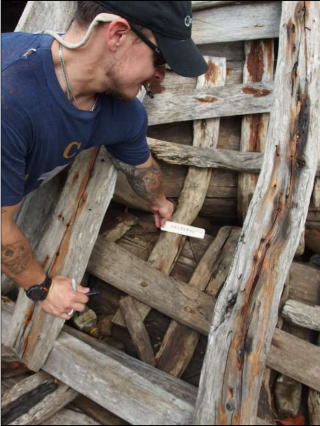
Author indicating the haligamu , or half-frame, Tongoni Village, Tanga Region (Photograph by Madeline Roth)
