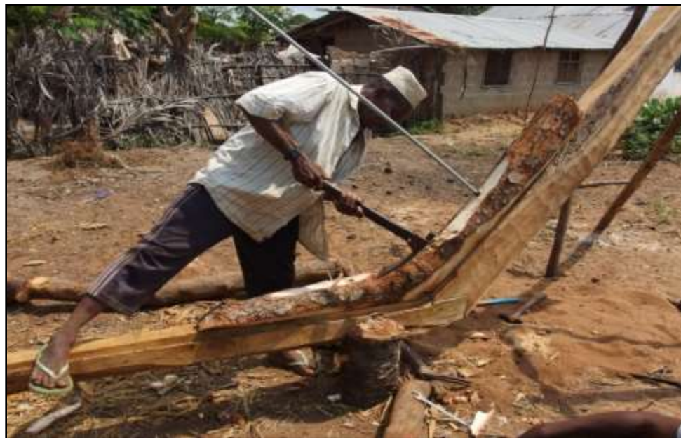
Figure 26: Mfundu Muddi forming the betana , or knee after securing it to the fashini , or stem post with a machined lag bolt, rabbet on keel visible, Tongoni Village Tanga Region (Photograph by Madeline Roth)
