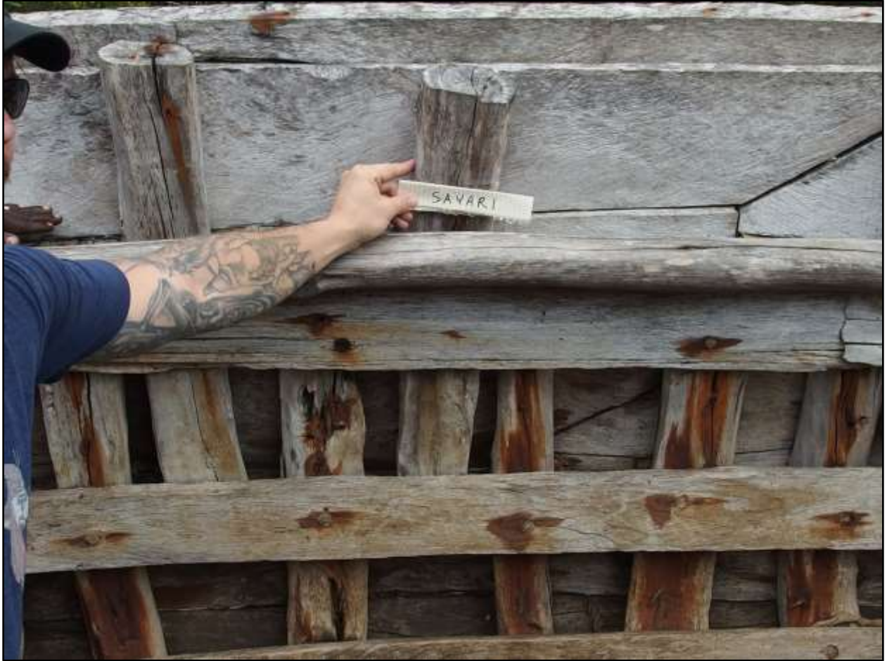
Author indicating the sayari , or half-frame component, Tongoni Village, Tanga Region (Photograph by Madeline Roth)
