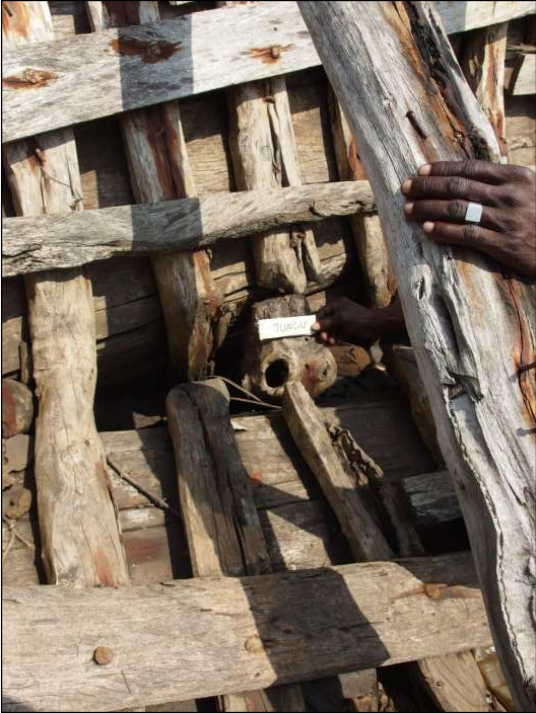
Author indicating the jungu , a stern keelson element, Tongoni Village, Tanga Region (Photograph by Madeline Roth)
