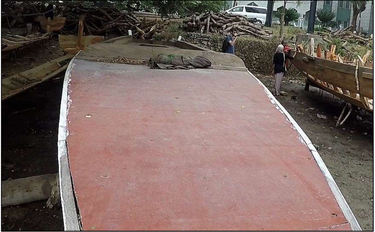
Image 40: Topside of mgwanda from stempost, illustrating covered cargo hold as seen on modern speedboats, Stone Town, Zanzibar
