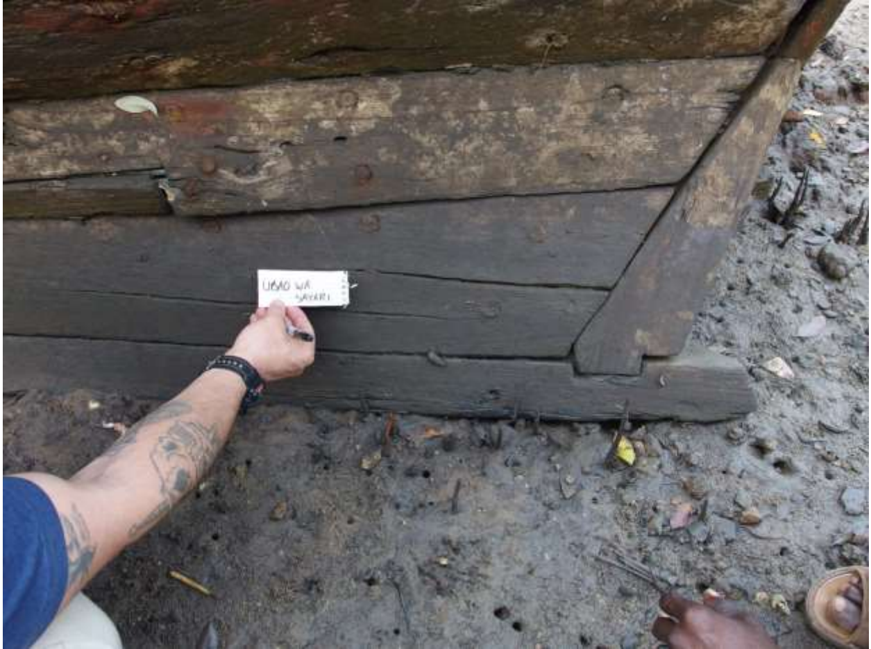
Author indicating the ubao wa sayari (wood of the planets) or lower hull planking towards transom, Tongoni Village, Tanga Region (Photograph by Madeline Roth)
