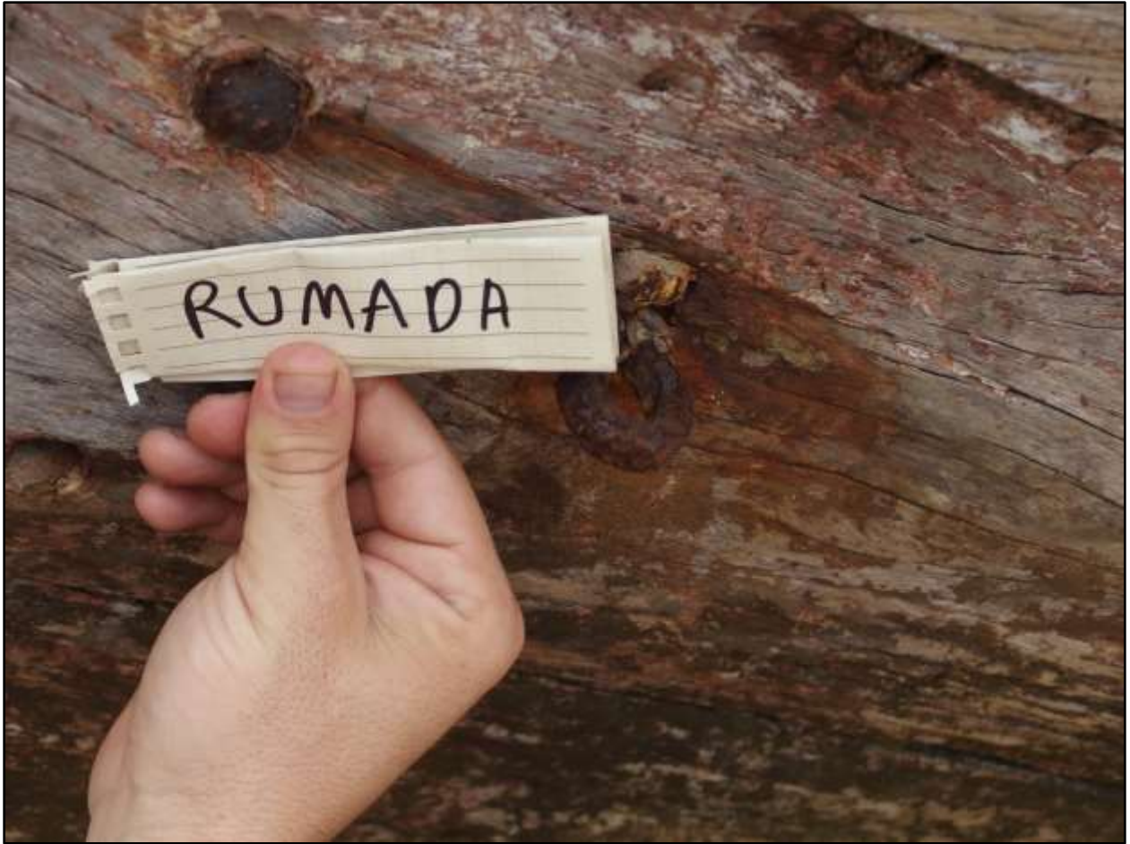
Author indicating the rumada , or gudgeon for rudder pintles, Tongoni Village, Tanga Region (Photograph by Madeline Roth)
