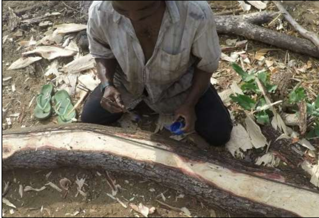
Figure 23: Mfundu Muddi outlines the formed rebar for the taruma using chalk paint before shaping the frame piece with his adze, Tongoni Village, Tanga Region (Photograph by author)
