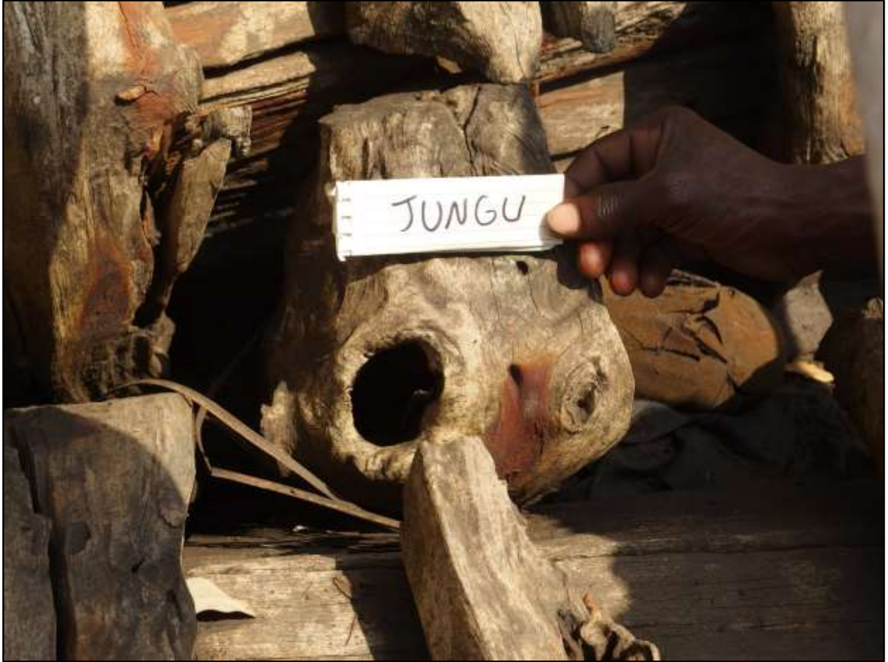
Author indicating the jungu , a stern keelson element, Tongoni Village, Tanga Region (Photograph by Madeline Roth)
