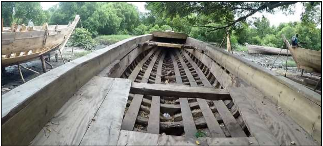
Image 39: Interior of mgwanda from the stern, displaying traditional framework including hand hewn Y-frames and riders despite modern hull design, Stone Town, Zanzibar (Photograph by author)
