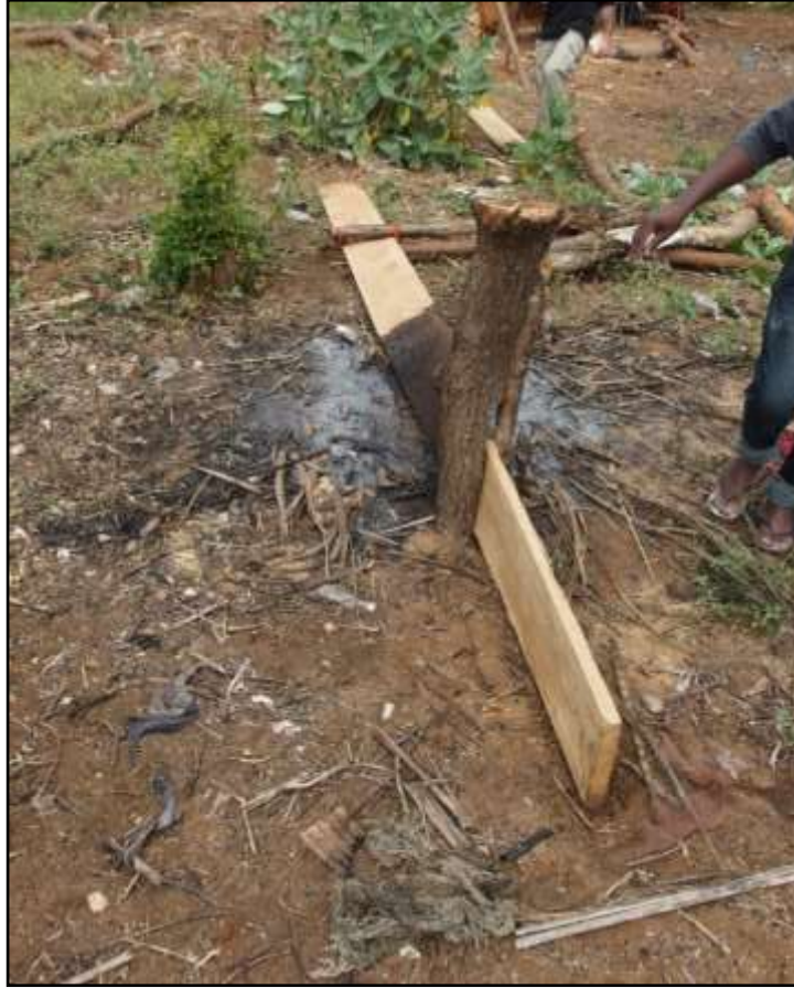
Figure 32: Hull planking being formed using kipindo , Tongoni Village, Tanga Region (Photograph by Madeline Roth)
