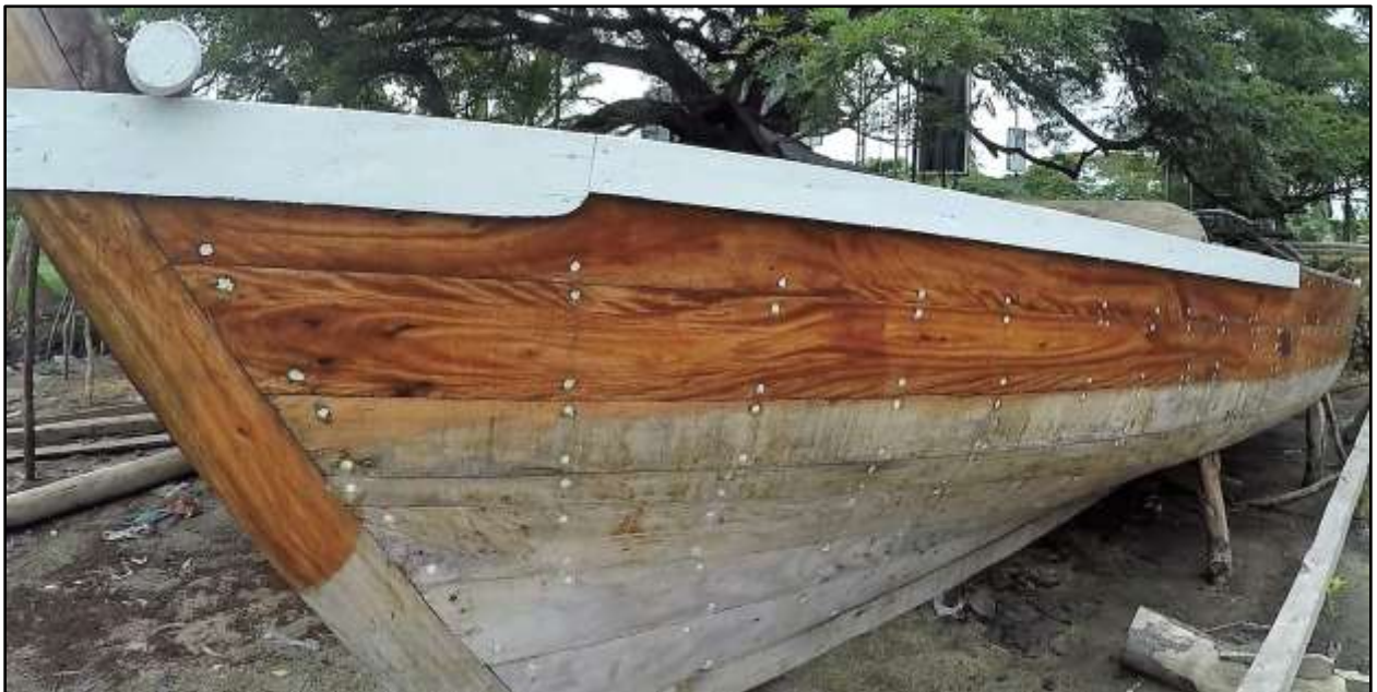
Image 37: Traditionally constructed speedboat, or mgwanda , Stone Town, Zanzibar (Photograph by author)
