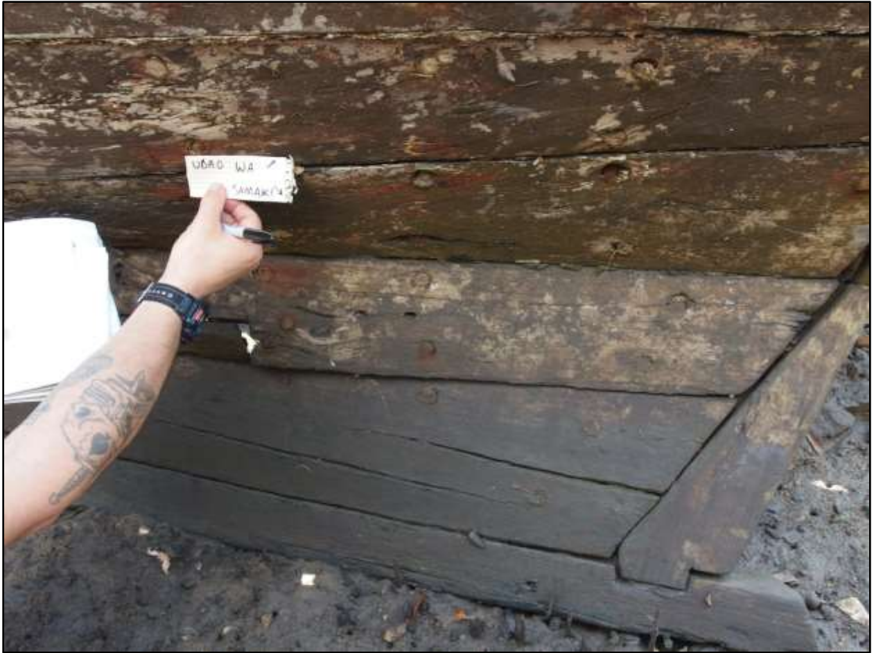
Author indicating the ubao wa samaki (wood of the fish) hull planking section toward transom, Tongoni Village, Tanga Region (Photograph by Madeline Roth)
