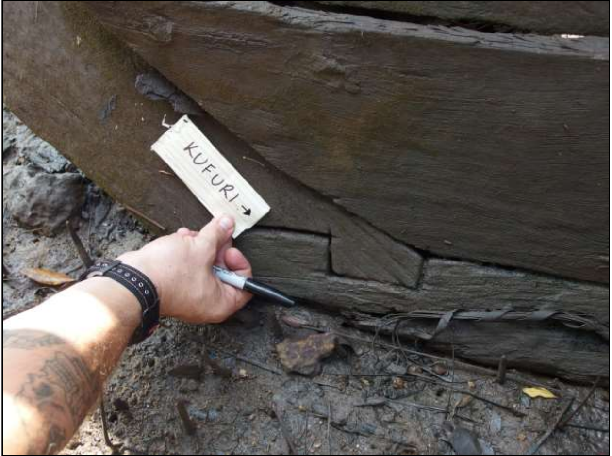
Author indicating the kufuri (lock), or the scarfed joint between the stem and the keel, Tongoni Village, Tanga Region (Photograph by Madeline Roth)
