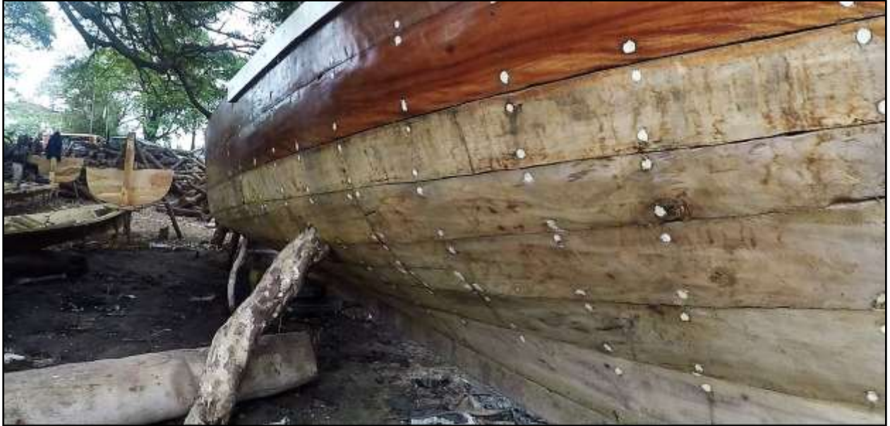
Image 38: Hull detail of mgwanda , illustrating its sleek profile and the use of concrete to cover nail heads, thus reducing drag, Stone Town, Zanzibar (Photograph by author)
