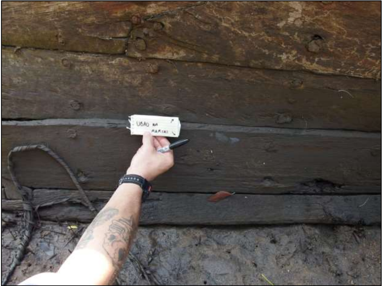
Author indicating the ubao wa mariki , or lower planking above garboard strake, Tongoni Village, Tanga Region (Photograph by Madeline Roth)
