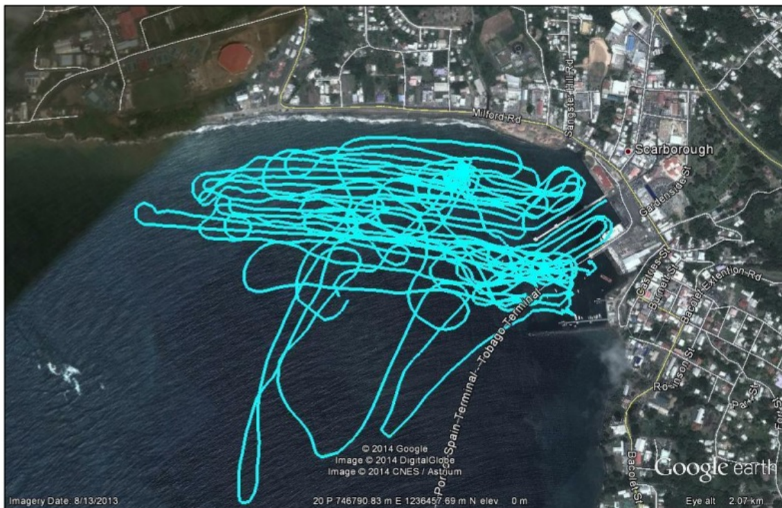
Figure 16. Survey lines tracking the area covered by the magnetometer survey (RBRP 2014).
