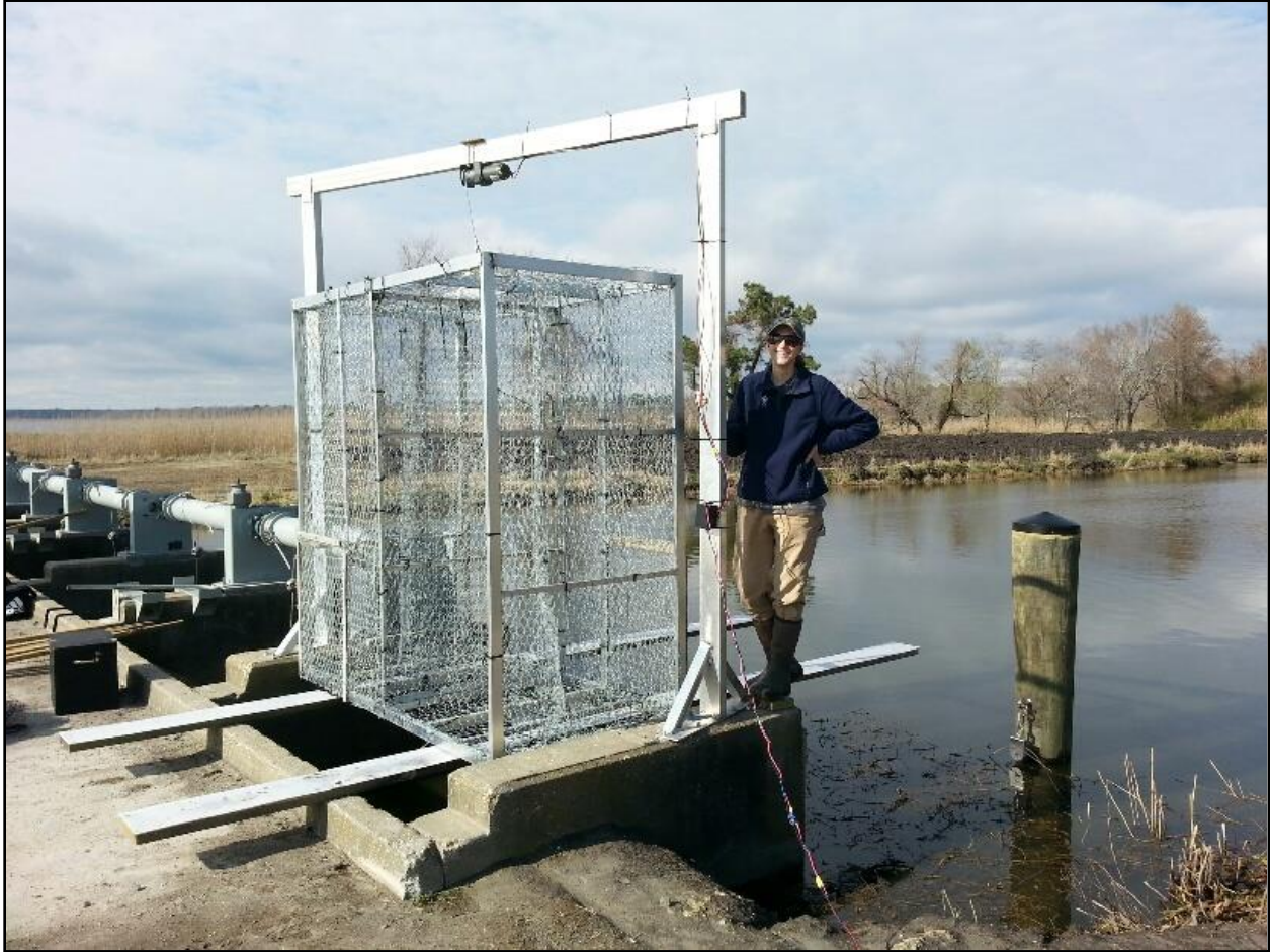
Figure 3.5. Author with lift system, electric winch, and custom-built dual-sided fish trap deployed in the side-opening gate during the 2015 and 2016 sampling periods at Waupoppin Water Control Structure, Lake Mattamuskeet, North Carolina.
