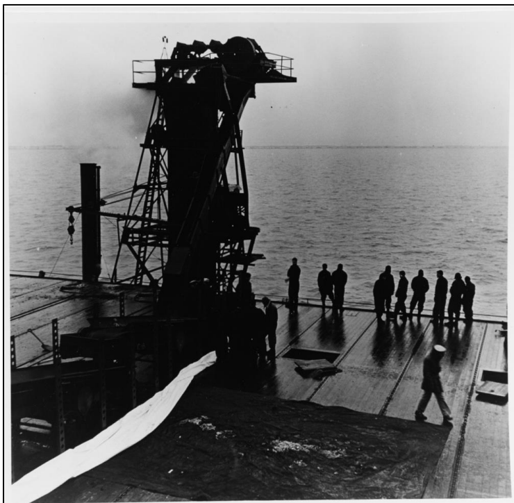
Figure 3.3. Collier alongside to refuel the training carrier, on Lake Michigan, December 1942. Note coal hoisting gear on the collier and conveyer belt system and coal hatches on the carrier's flight deck (Photo, Lieutenant Wayne Miller, USNR. Courtesy of Naval History and Heritage Command).
