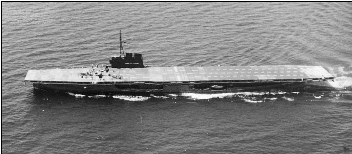
Figure 3.5. USS Sable steel decking differences evident aft of conning tower, June 1945 (Courtesy, Naval History and Heritage Command).
