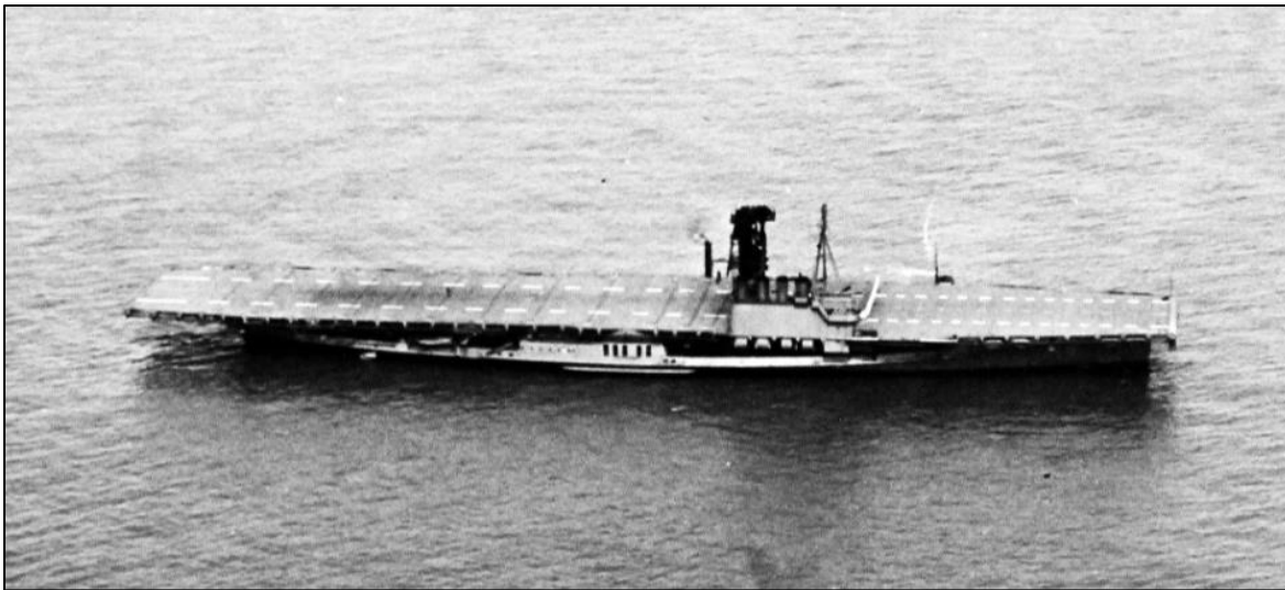
Figure 2.8. USS Wolverine on Lake Michigan, with no forward anchor staffs visible, April 6, 1943 (Courtesy, Naval History and Heritage Command).
