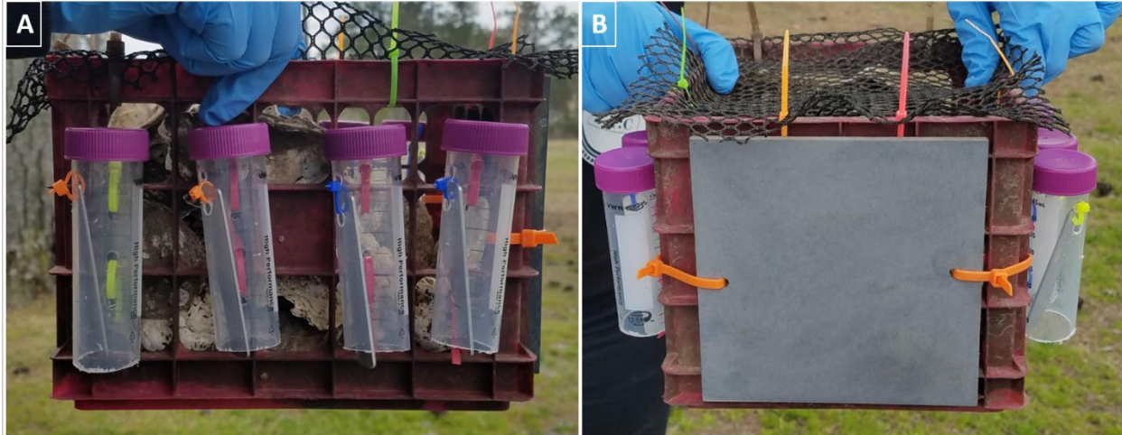
Figure 1: Deployment crates used to attach protected metal coupons (A) and biofouling plate (B).
