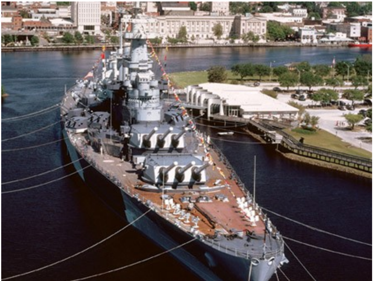
Figure 29. Image showing the mooring system installed to keep USS North Carolina in place.
