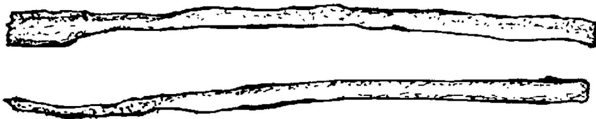
FIGURE 46. Crow (NS2.A6a.1b) excavated from Port Royal, measures 18.9 in. long. The round stock measure approximately 0.75 inches while the flattened end is 1.1 in. wide and 0.25 in. thick (Franklin 1992:97).
