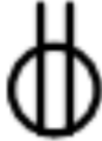
Figure 4.1: Scanned Image of Outlet Symbol (enlarged)
