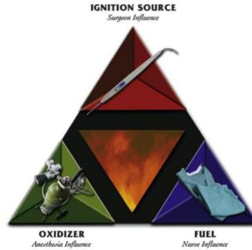
**Anesthesia is primarily responsible for managing the oxidizer component of the fire triad (O<sub>2</sub> and N<sub>2</sub>O)<sup>1</sup>**
