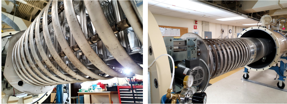
Figure 1.1: Shows the state of the accelerator when brought up to air. In each panel there is evidence of a black substance on the surfaces, which was caused by a failure in the terminal chain pulley bearing.
