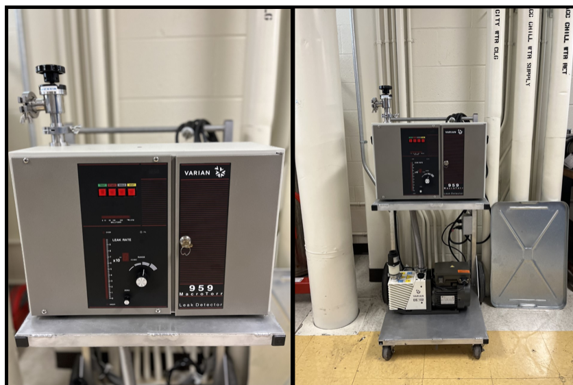
Figure 1.3: The helium detector, this device is fitted with both a rough pump and turbo pump to pull low vacuum for any device it is connected to. The left panel shows the control interface for the detector, and the right panel gives a full view of the detector.
