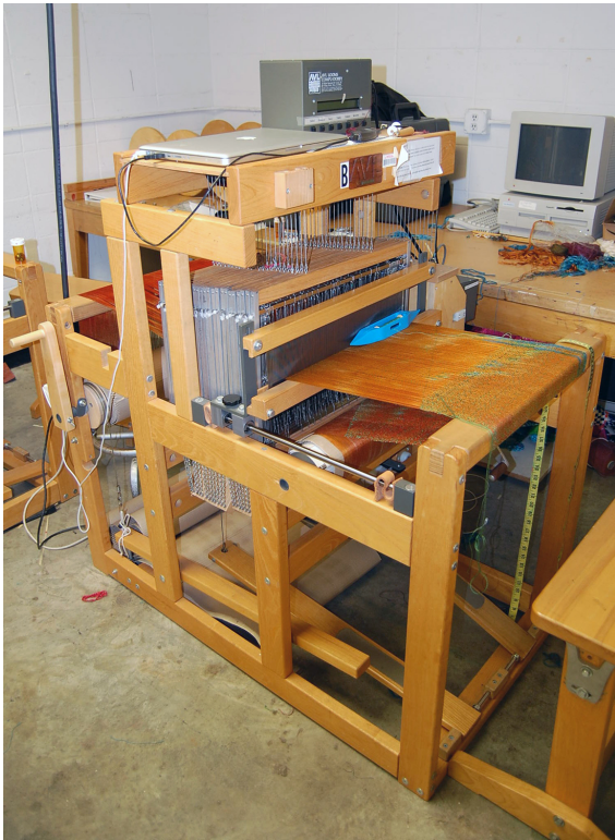
Figure 5. AVL Compu-Dobby Loom.
