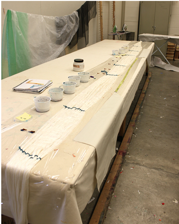
Figure 3. Warp stretched out ready to be painted.
