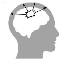
Figure 5: A representation of volume conduction artifact. Multiple electrodes may pick up on the same source activity.
