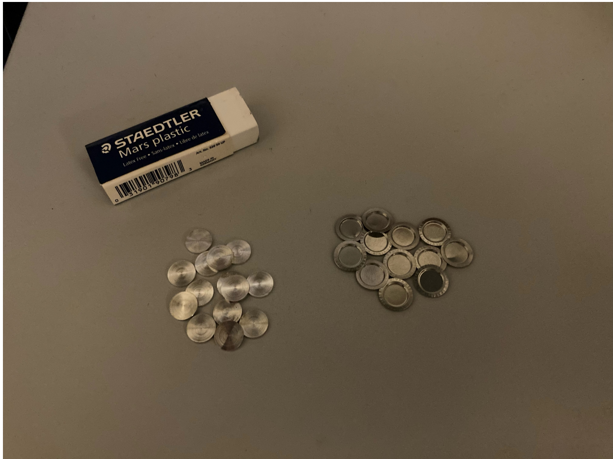
Figure 3.2: Image of the Risø TL/OSL DA-20 luminescence reader cups with eraser for scale. The stainless-steel disks (left) are 9.7 mm in diameter and the stainless-steel cups (right) are 11.65 mm. Sediment is adhered to the disks or cups and placed into the sample carousel for measurement.
