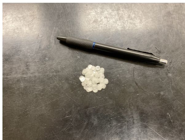
(c) Luxel dosimeter chips were created using a single-hole punch.
