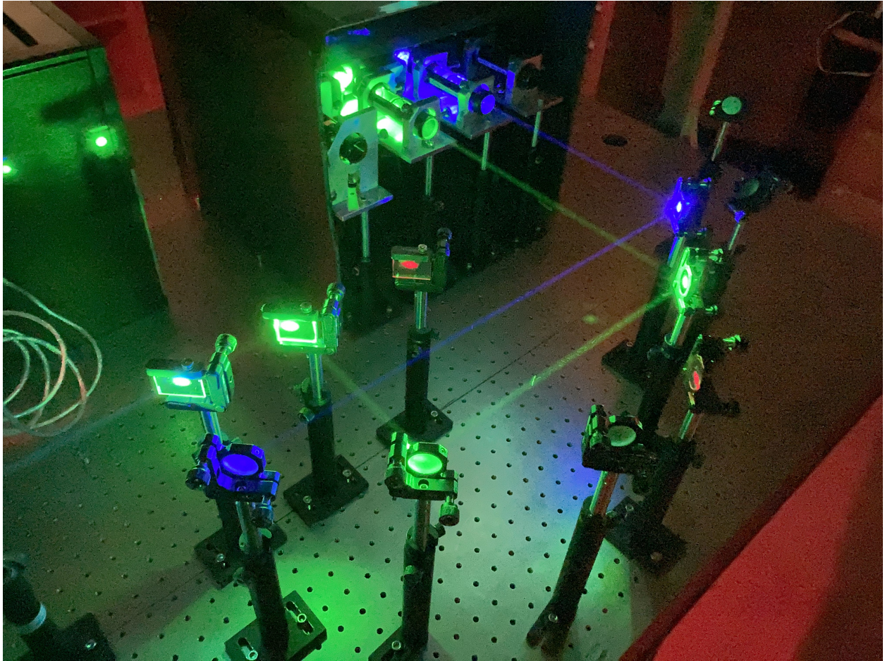
Figure 5.3: Image of LuCIDD’s stimulation unit. All visible lasers were switched on for the photo, but only one will be used at a time during focusing and measurement. Only the high-power blue and green beams can be seen passing through the air.
