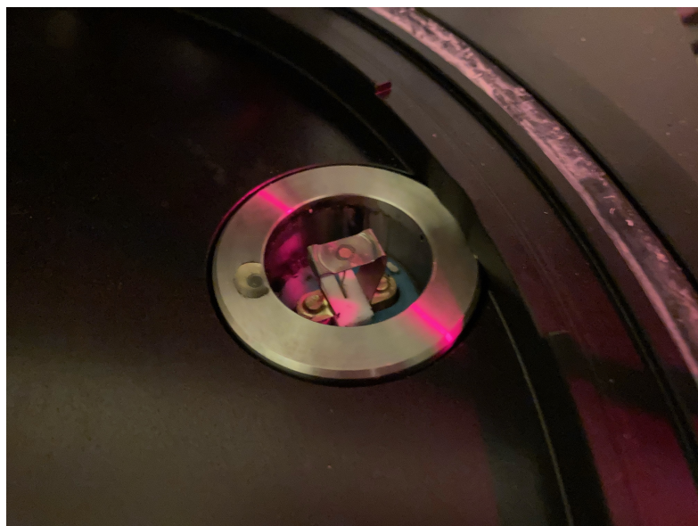
(a) Image of the Risø's heater element. It is able to lift the sample to the measurement area and raise the temperature up to 700°C. The heating element is useful for both low temperature heating during optical stimulation as well as high temperature thermoluminescence stimulation.
