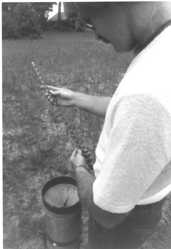
Figure 3-4. Standard rain gauge. The rain gauge should be in a location in which surrounding trees cannot influence its reception of atmospheric moisture.
