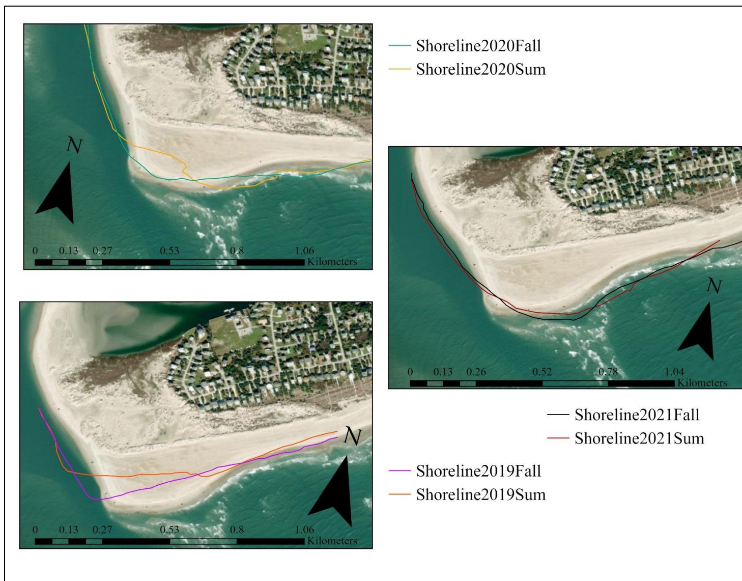
Figure 30. The base aerial image is from 07/2023 and sourced from Google Earth. Maps of shorelines digitized in ArcGIS Pro version 3.0 using Geodynamics' topo/bathymetric data. The three maps show the spatially varying shoreline movement from Summer to Fall 2019, 2020, and 2021.
