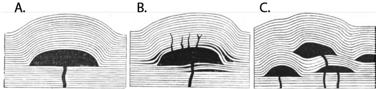
Figure 6: Schematic sketches of idealized laccoliths (Modified from Gilbert, 1877). (A) A basic laccolith. (B) A laccolith with associated dikes and sills. (C) Multiple laccoliths in one location.
