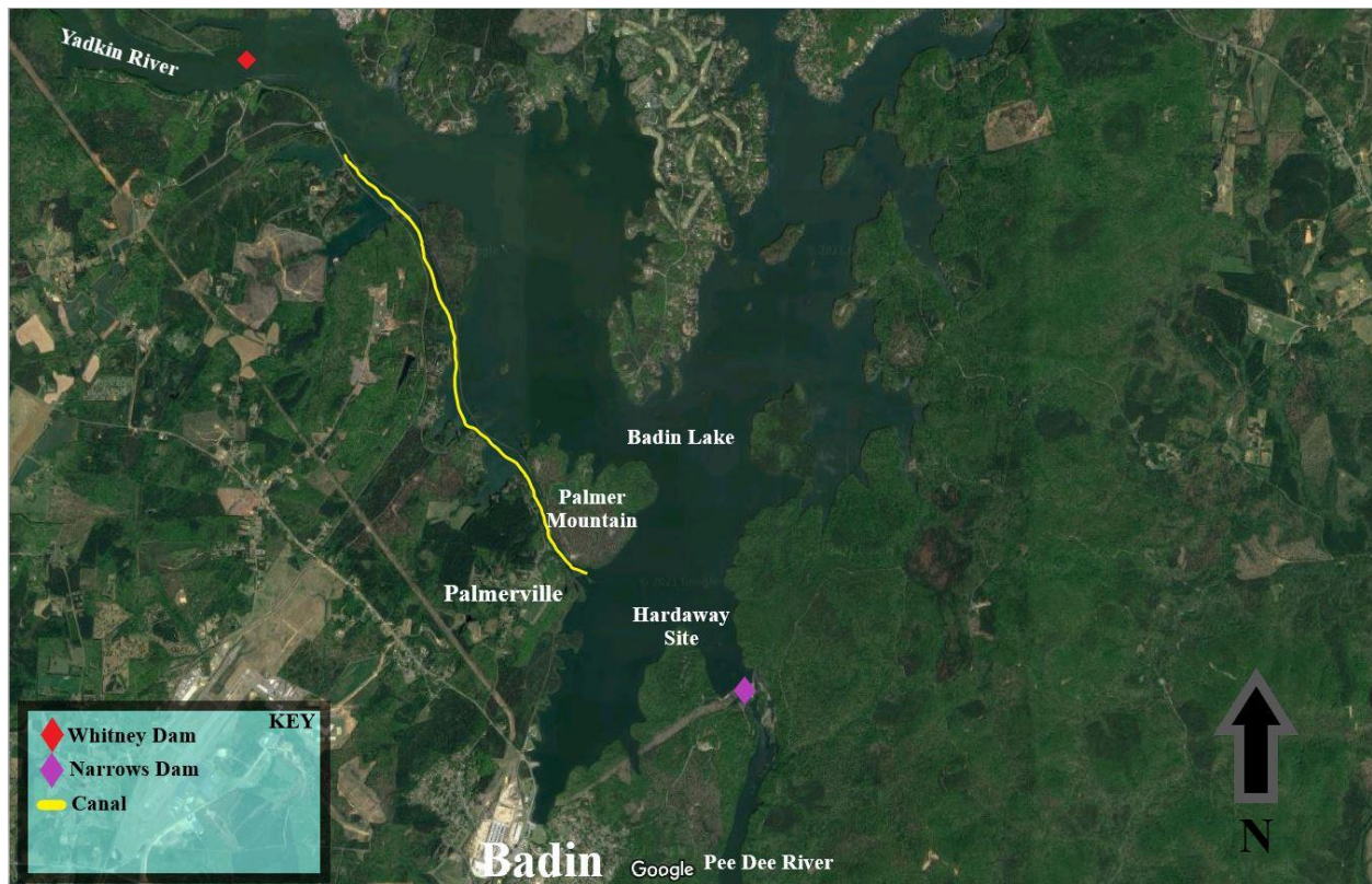
Figure 2. Satellite imagery Badin Lake region showing the approximate location of Whitney Dam ruins, the canal remnants, and present Narrows Dam (Photo from Google Maps).
