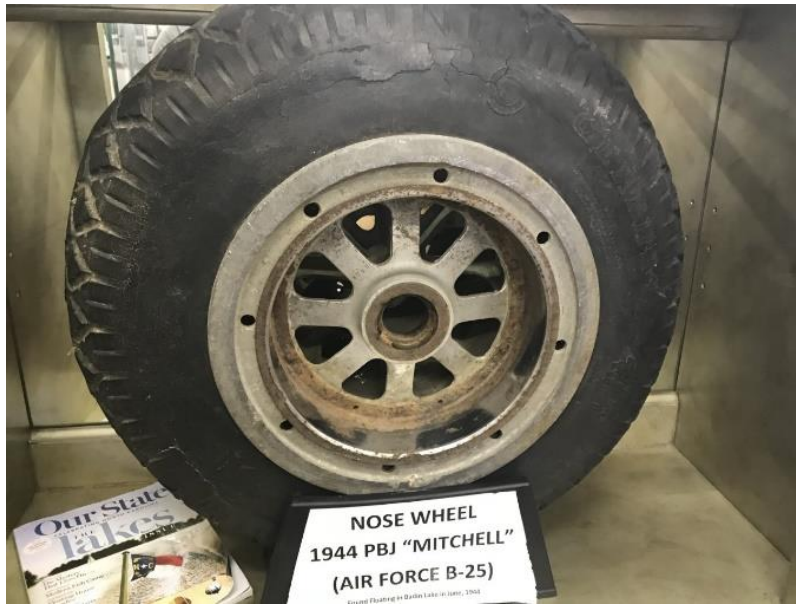
Figure 34. Nosewheel starboard side from B-25 Landing Gear (Photo by P.Smith).
