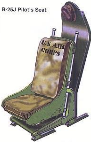
Figure 28. Illustration of B-25J variant pilot and co-pilot seats (Drendel 1997:64).
